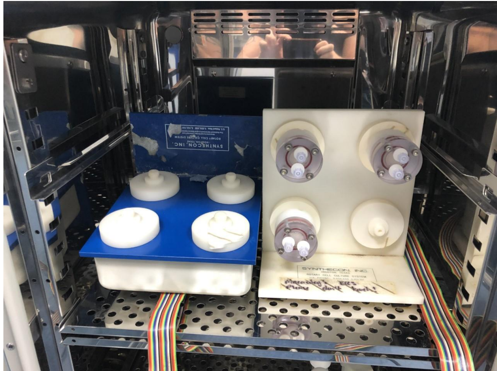
Figure 1.2.1.1: The 2D Clinostat known as the Rotating Cell Culture System (RCCS). The RCCS is capable of rotating up to four individual cell culture vessels. These cell culture vessels carry media containing cells in 1 mL, 2 mL, 10 mL or 50 mL formats. The cell culture vessels come in two varieties, disposable and autoclavable. The vessels compose of two Luer Lock syringe ports for small additions or extractions to the cell media and a larger fill port for ease of filling and emptying. The rear of the vessels composes of a gas exchange membrane to allow the diffusion of gases. The vessels rotate clockwise at independent or synchronous speeds [119]. The schematic shows the parts of the RCCS and names the individual components. The photo shows the RCCS set-up used for the studies in this thesis with one RCCS being in a horizontal 'control' orientation and the other RCCS in the '0 g' analogue orientation. Attached are 2 mL autoclavable HARV vessels.
