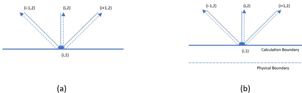
Fig. 3-2 Schematic of (a) standard bounce-back scheme and (b) half-way bounce-back scheme
