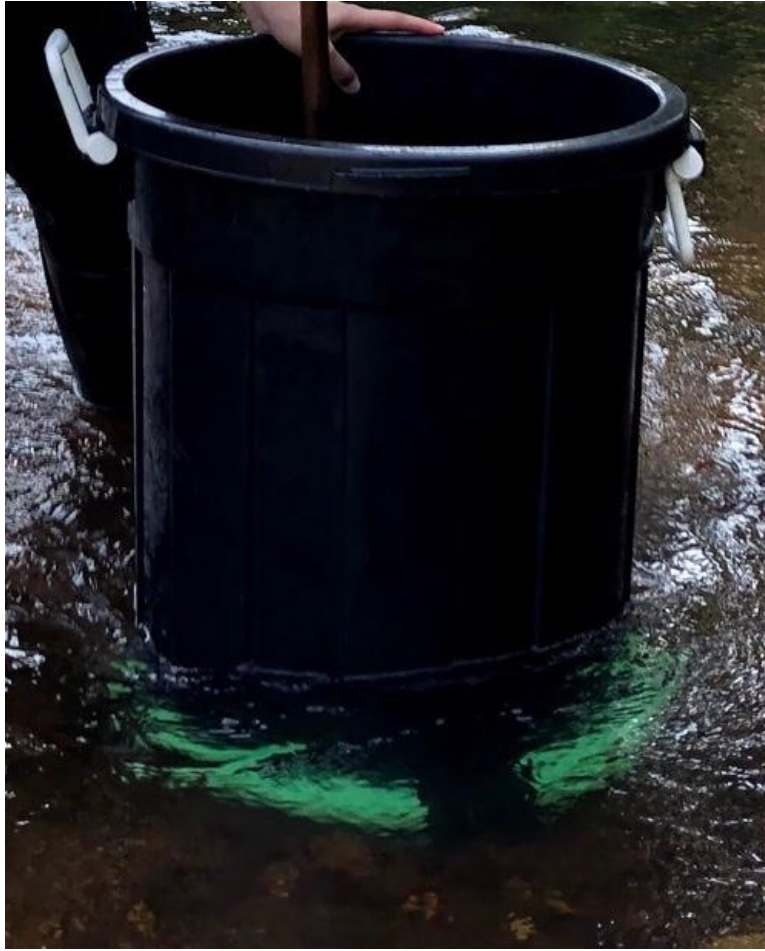
Figure 3.2. Open-ended truncated cone used for sediment sampling.
