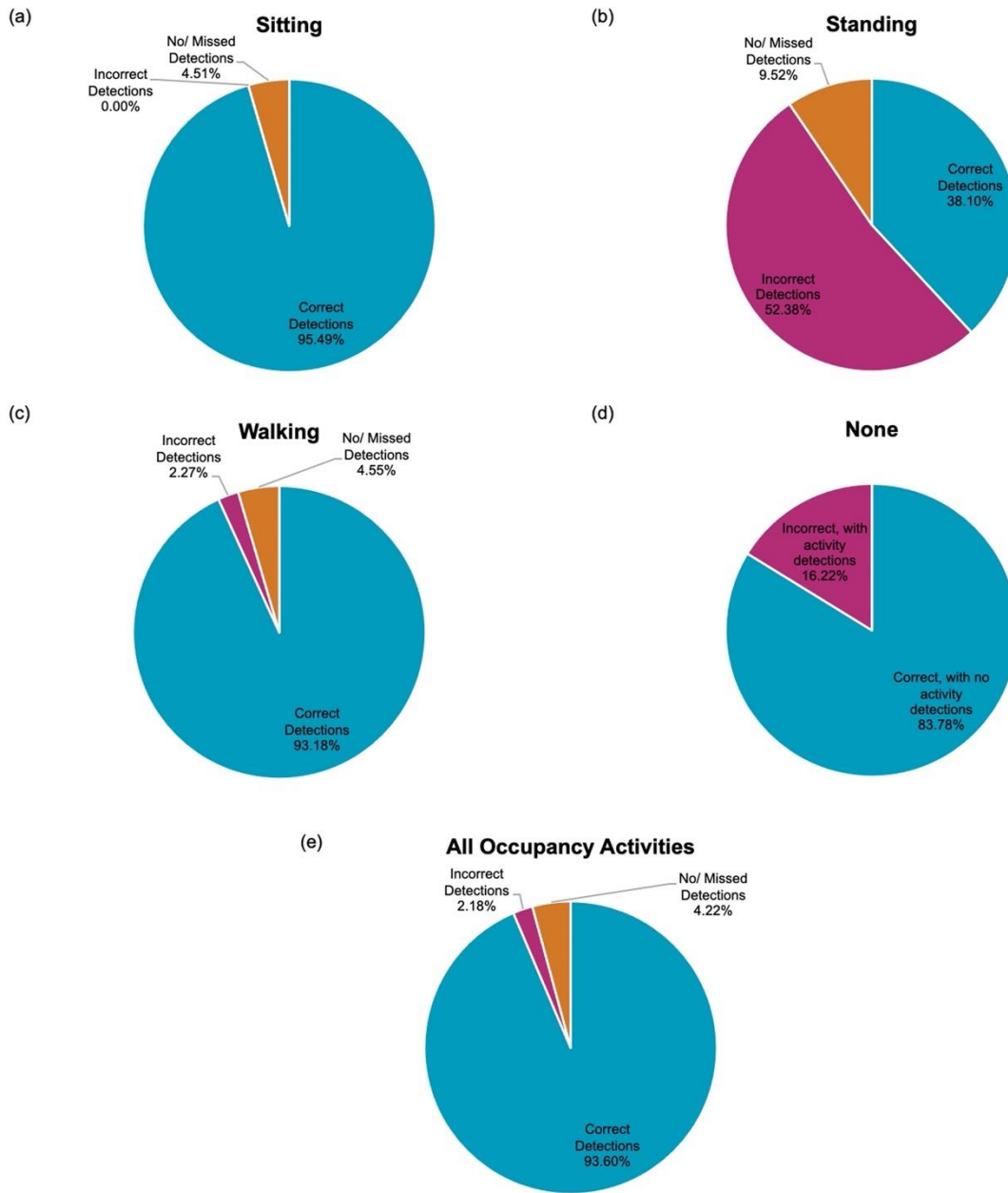
Figure 6-10. The detection performance of occupant activities during Experimental Test 2 for combined detections.
