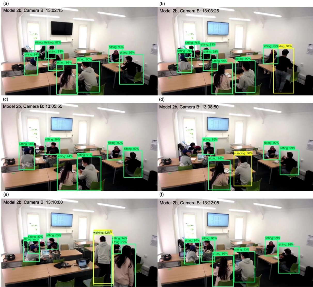
Figure 4-33. Snapshots of occupancy detection and recognition during key stages of the experimental Test 4 using Model 2b.
