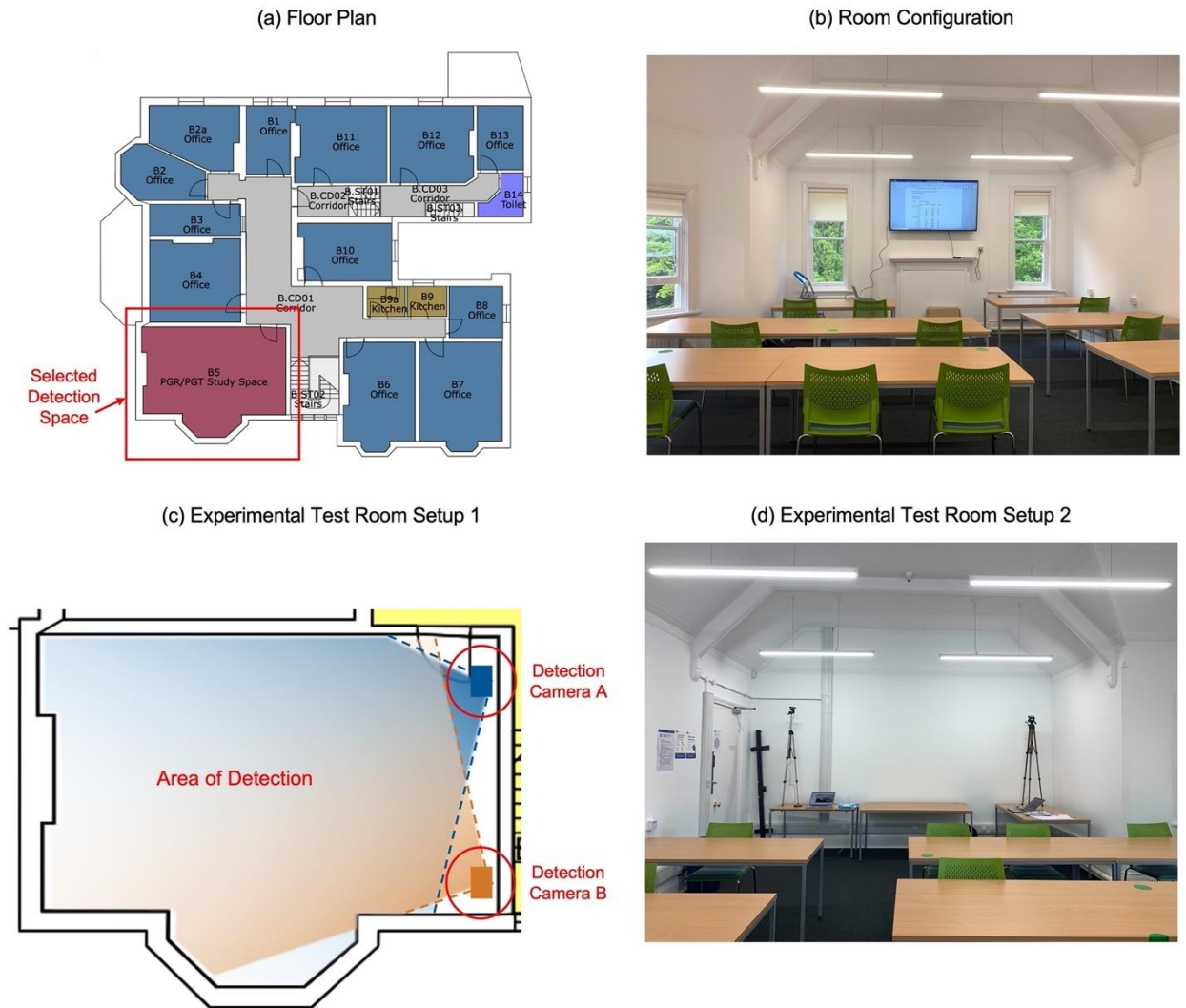
Figure 4-19. Paton House at the University of Nottingham applied in Experimental Tests 1 and 4. a). Floor plan of the first floor of the building with the room configuration in (b). Setup for the experimental tests in (c), and (d).
