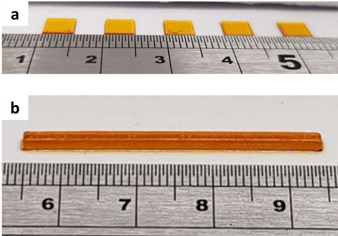
Figure 4.6: Examples of IJP printed outcomes for (a) 100-layer 5 x 5 mm square patterns and (b) 40 x 2 x 2 mm implant exemplar. Ruler scale (cm).
