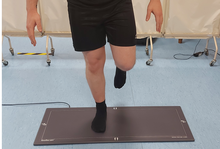
Figure 4.5: Image of the pressure force plate used to measure distance moved and ellipse area of centre of pressure to assess balance
