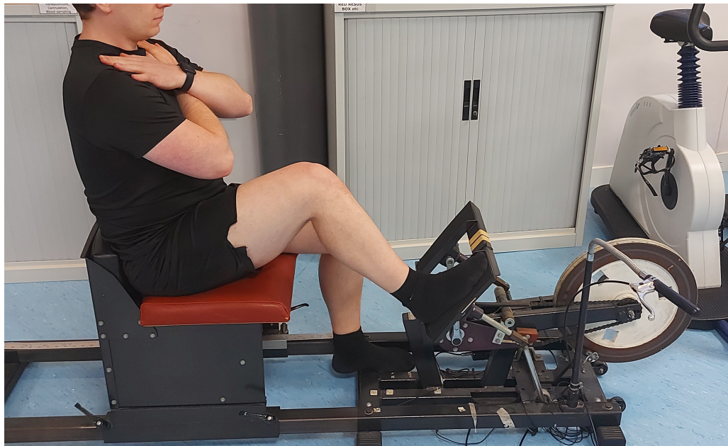
Figure 4.4: Image of Nottingham power rig, as used to test leg extension power
