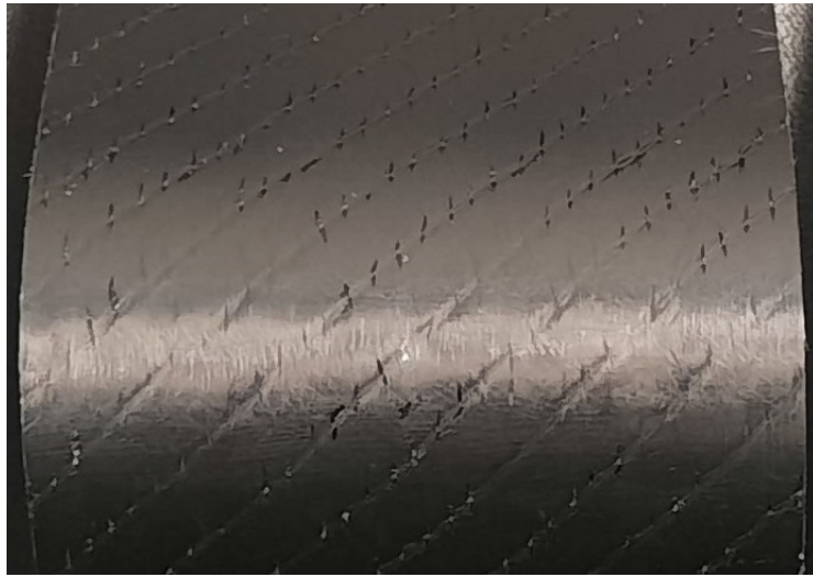
Figure 3.16: Pinholes at the tool side of the AS 16 specimen 2.
