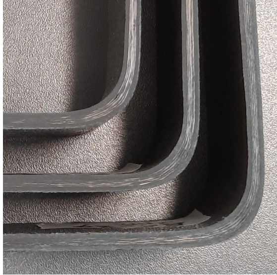
Figure 3.18: Corner thickening of the BF 16 specimen group.
