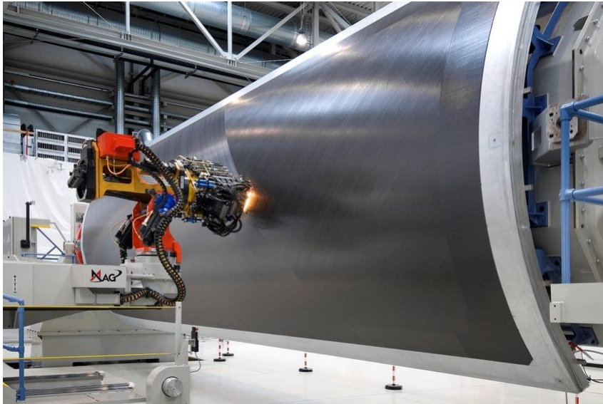
Figure 1.8: Automated Tape Laying (ATL) on an Airbus A350 upper shell fuselage skin section at the premises of Premium AEROTEC GmbH [8].
