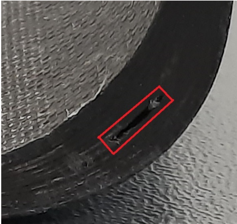
Figure 3.14: Fibre bridging of the ST_{16} specimen 3 manufactured from the aluminum tool.
