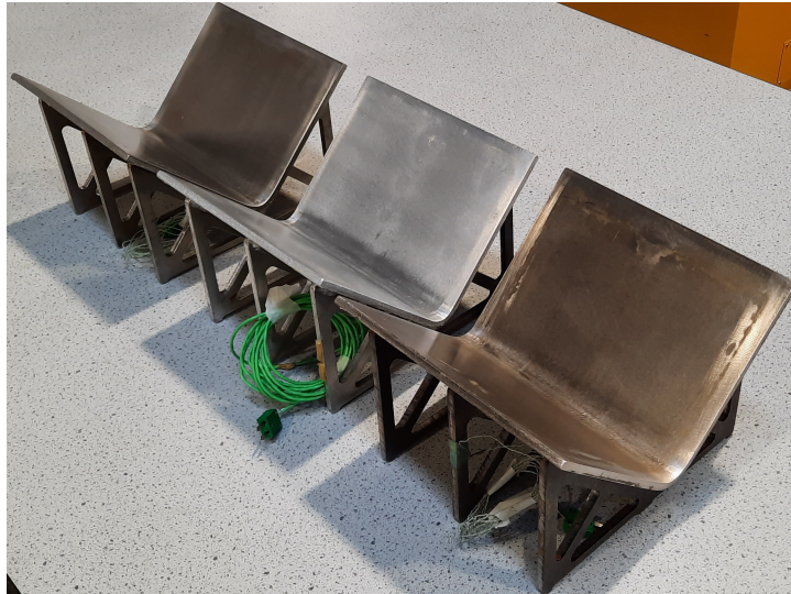
Figure 3.4: The three tools used to manufacture the specimens (From top to bottom: Steel, Aluminium and INVAR).
