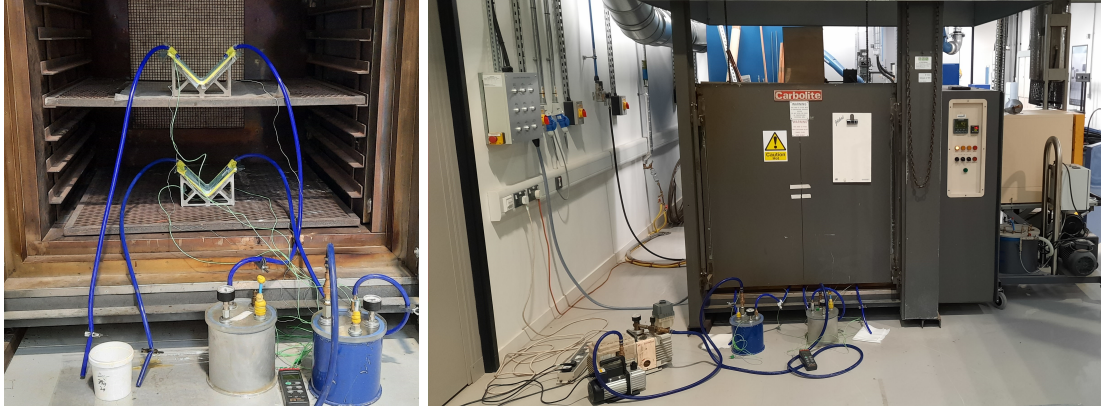
Figure 3.10: Arrangement of the equipment before (left) and during (right) the curing cycle. The oven used to preheat the resin is the small one next to the oven used to manufacture the specimens.
