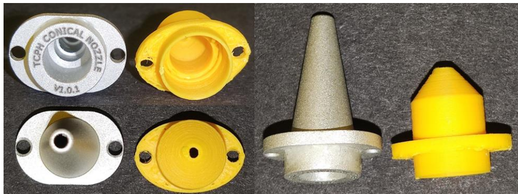
Figure 5.8 Side to side comparison of existing nozzle cap ( grey ) and PLA printed custom made nozzle cap ( yellow )
