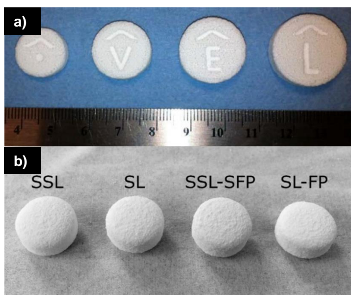
Figure 1.3 Examples of binder jetting printed tables. a) Aprecia's Spritam® tablets in all of their four strengths [45]; b) SLS printed tablets utilising different grades of hydroxypropyl cellulose [105]
