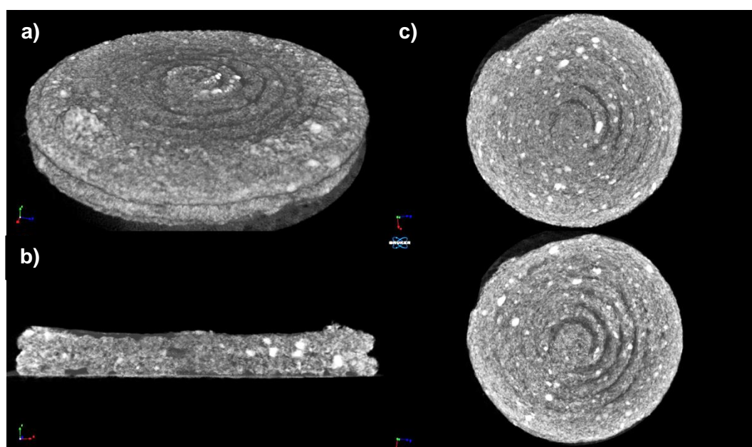
Figure 3.3 Micro-CT scan of a solid FR printed tablet. a) top view, b) vertical cross section, c) horizontal cross sections at different heights of the tablet
