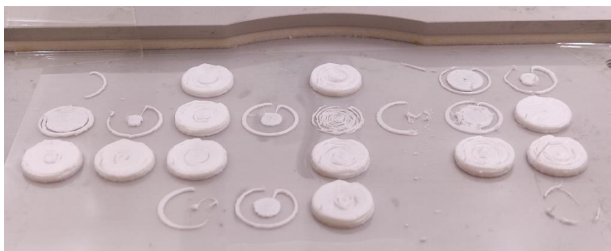
Figure 5.11 Successful printing attempts of eutectic printed tablets
