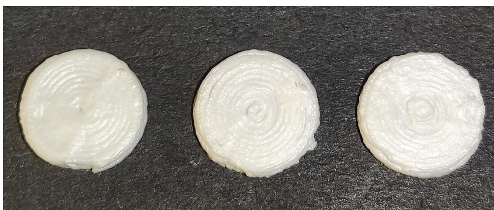
Figure 5.20 3D printed tablets used for dissolution
