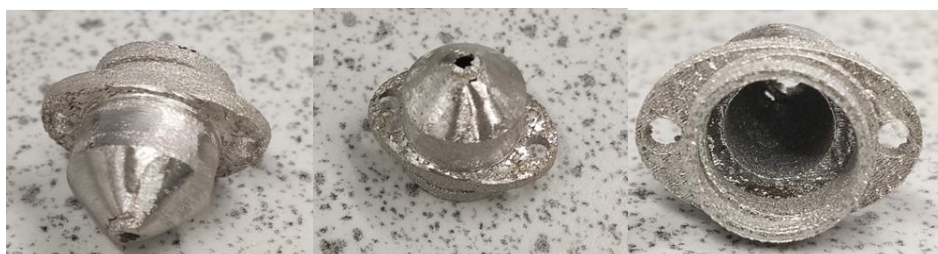
Figure 5.10 Different angles of laser powder bed fusion printed nozzle cap
