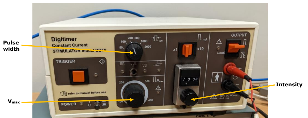
Figure 2.8. The Digitimer Constant Current STIMULATOR model DS7A.
