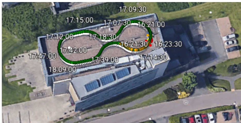
Figure 8.1: Reference solutions on Google Earth. Green, yellow and red points standard for fixed, float and single solutions respectively.
