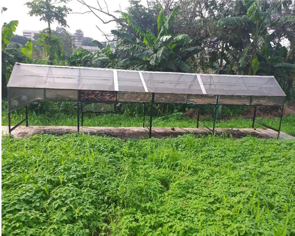
Figure 5.5: Solar dryer filled with some cocoa pod husk
