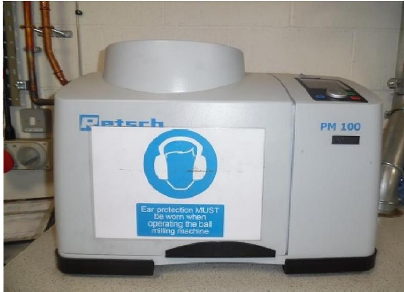
Figure 3.2: Retsch Planetary Ball Mill PM 100
