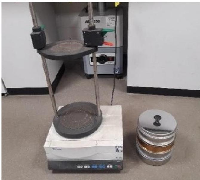
Figure 3.3: Retsch Electromagnetic Shaker AS 200 with sieve mesh on the side
