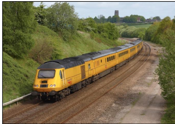
Figure 3.5 Track recording vehicle (after [72])
