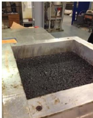
Figure 41. Resulting Asphalt slab in 305 x 305mm mould
