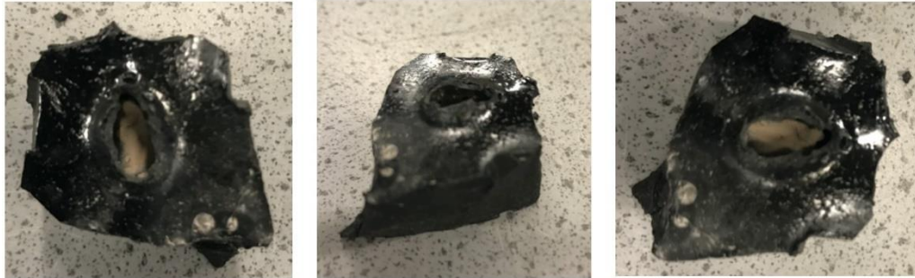
Figure 101. Image of Internal detritus cake for Test 5 (T5)
