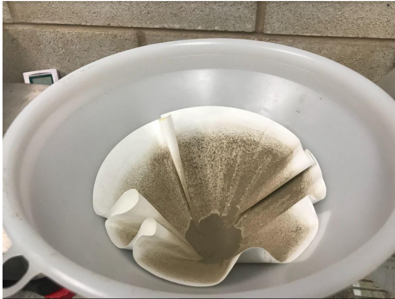
Figure 57. Detritus caught in cracks on filter paper in funnel.
