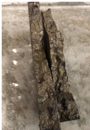
Figure 56. Crack face of slice showing dirt caught in cracks.
