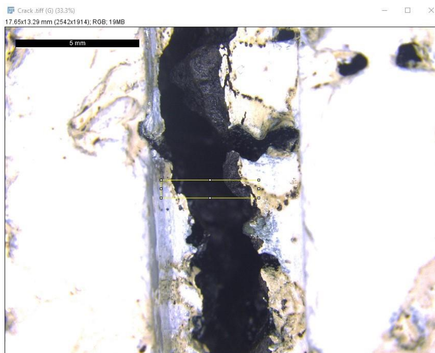
Figure 70. Image of crack showing ROI
