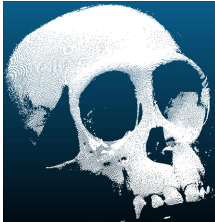
Figure 1.1 Example of a fringe projection measurement. A measurement of a skull from the Zoology collection, School of Life Sciences, University of Nottingham, Thomas Hartman. Each dot is a single point within the point-cloud.
