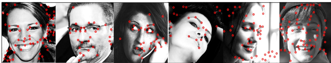
Figure 3.7: Visual examples of generic keypoints detected by SuperPoint [40] on facial images.
