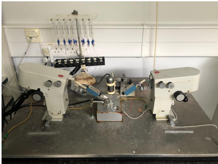
Figure 2.7.1.1: TEVC setup. A transfected oocyte is placed in the perfusion chamber where it then exposed to varying concentrations of drugs and physiological solution ( Xenopus ringer) through a multi-channel perfusion system. The microelectrodes were connected to the headstages which were connected to geneclamp 500B amplifier and the digidata A/D converter. This setup was connected to a PC.
