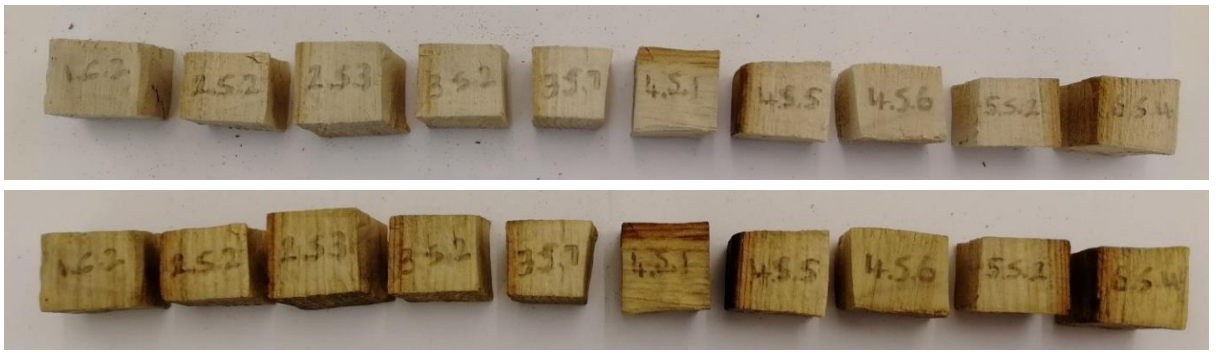
Figure 3 (a) Photographs of treatment group 1 (TPA6) before (top) and after (bottom) treatment. Specimens became noticeably darker, with a yellow tinge. (b) Photographs of treatment group 2 (TPA7) before (top) and after (bottom) treatment. Specimens were similar to those treated with TPA6.
