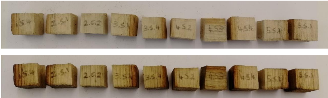
Figure 95. Photos of treatment group 1 (TPA6) before (top) and after (bottom) treatment. Specimens became noticeably darker, with a yellow tinge.
