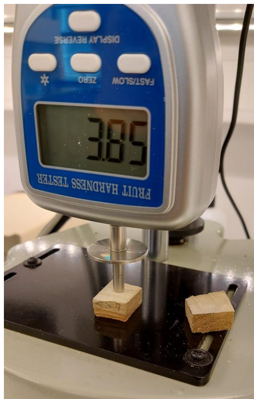
Figure 77. The tangential surface of a treated archaeological wood specimen being analysed with the fruit penetrometer (top left and right). The core of a treated specimen being analysed (bottom).
