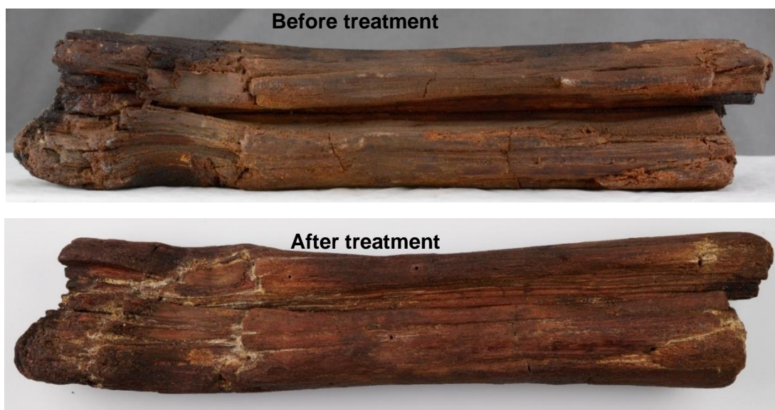
Figure 117. Wood fragment from the Oseberg collection before and after retreatment by injection with PDMS-OH (36,000 Da) in turpentine (5% concentration) and \text{Ca}(\text{OH})_2 nanoparticles. The fragment had originally been treated with alum and linseed oil after excavation. The fragment was injected for a period of 11 days and then left to dry for 34 days (Museum of Cultural History, University of Oslo).
