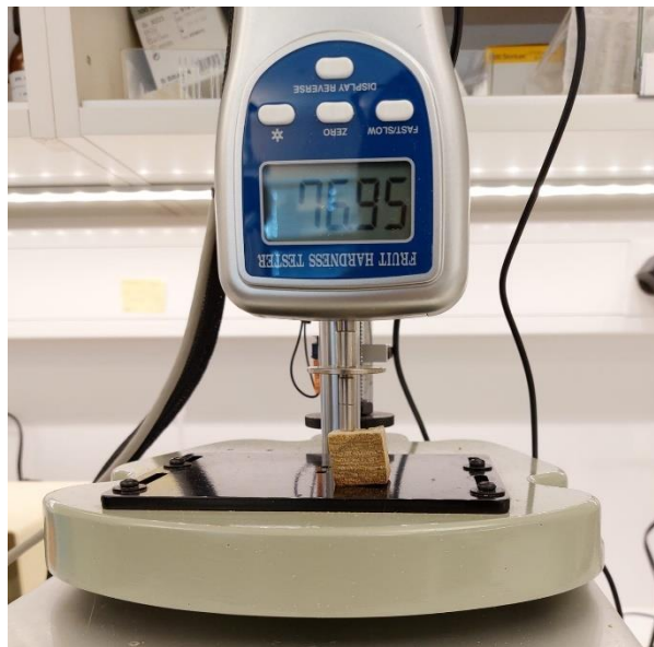
Figure 76. Photos showing the fruit penetrometer set-up, with a sound wood specimen (top) and an archaeological wood specimen (bottom).
