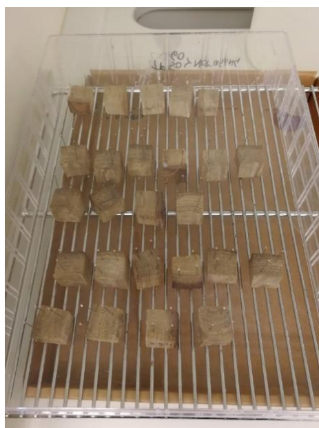
Figure 70. The treated cubes drying in the fume-hood after two weeks of immersion
