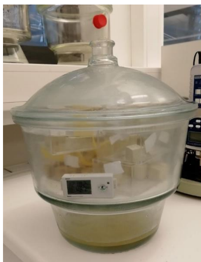
Figure 71. A photo depicting the conditioning set-up in a desiccator.
