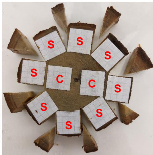
Figure 66. The original wood log which was used to cut the slices, numbered 1 to 6 (top) and the process of sawing off the specimens from one of said slices (bottom). The graph paper shows squares which are 2 x 2 cm 2 . Each specimen is labelled S or C, indicating if it was cut from the surface (S) or the core (C) of each slice.
