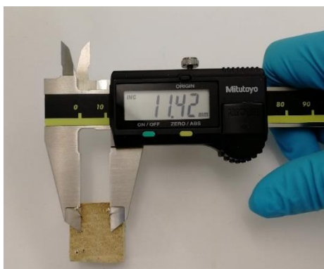
Figure 72. A photo depicting the method of measuring dimensional change with reference pins and electronic callipers.
