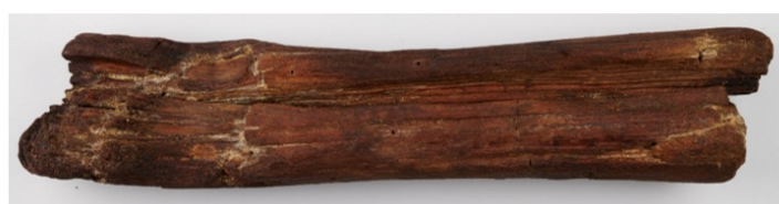
Figure 2. Wood fragment from the Oseberg collection before and after retreatment by injection with siloxane PS36000 in turpentine at a concentration of ~5% (50 g/L). The fragment had been originally treated with alum and linseed oil shortly after excavation in 1904.
