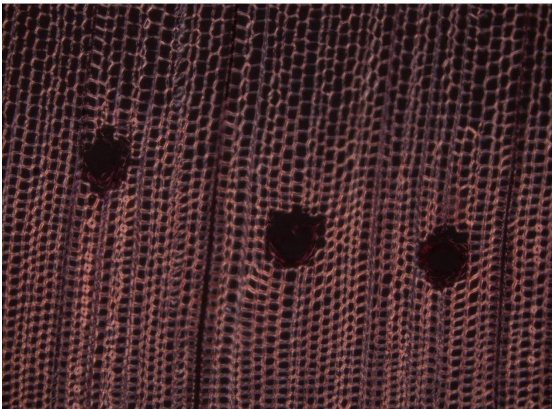
Figure 85. Transverse face of archaeological pine (top) and sound pine (bottom), as seen under the light microscope using a magnification of 200x. A loss of birefringence was observed under crossed polars when compared to the fresh wood, indicating the degradation of cellulose.
