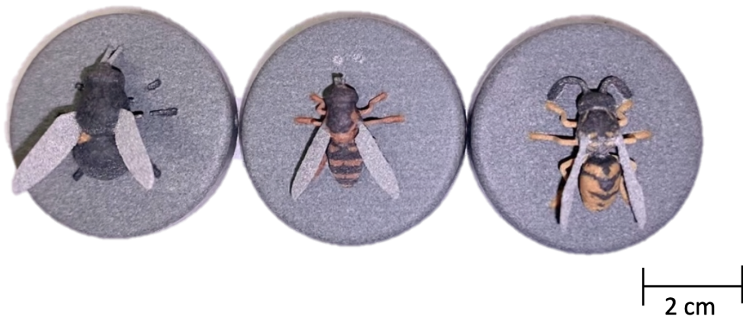
Figure 2: 3D printed models of Mesembrina meridiana (Left), Syrphus ribesii (Centre) and Vespa vulgaris (Right), prior to being removed from the base plate.
