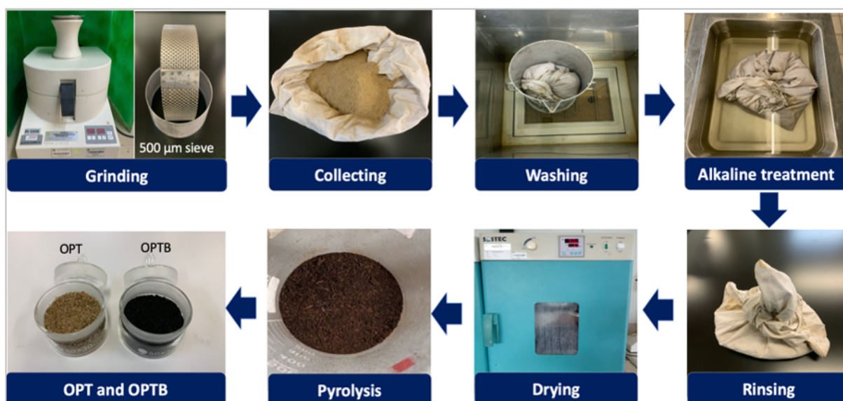
Figure 7.15: Different stages involved in the preparation of OPTB.
