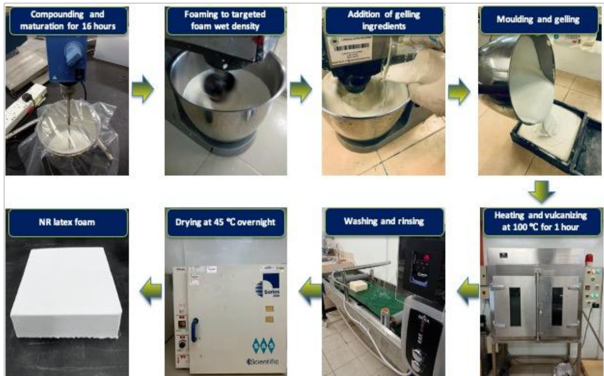
Figure 5.8: The different stages involved in the fabrication of SpNR latex foam.
