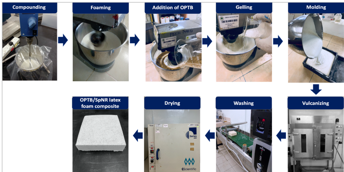
Figure 7.19: The steps involve the fabrication of the OPTB/SpNR latex foam composite.
