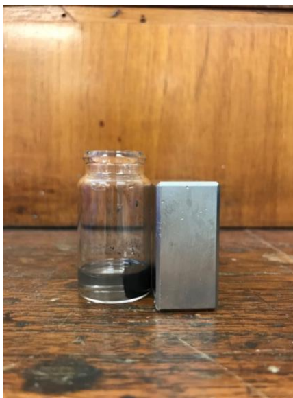
Figure 6.4. Photograph of magnetic catalyst being separated using a magnet.
