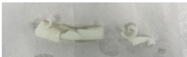
Figure 4.32: Hydrogel A after 5 days in PBS at 37°C.
