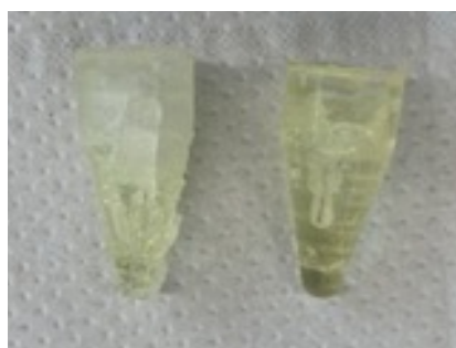
Figure 4.37: Successfully cured hydrogel U formulations produced in the silicone mould prototype.
