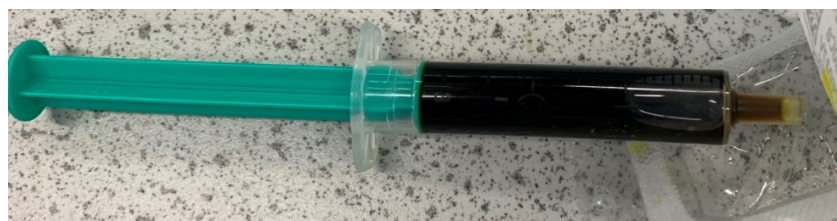
Figure 4.22: Hydrogel ink after use in the BMF nanoArch S130 printer. It had become black and unstable.
