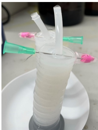
Figure 4.11: Adjustment made to the silicone moulds to produce hydrogels with thicker walls. The extrusion of the mould was stretched out and a needle placed through it and rested on the top of the mould.
