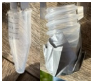
Figure 4.34: Construction of the mould for producing silicone moulds for hydrogels. The centrifuge tube was placed inside the corrugated plastic tubing and the base of the tubing was sealed with duct tape.
