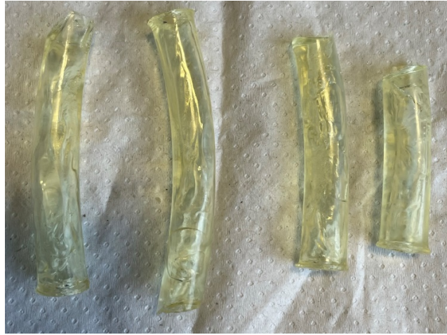
Figure 4.43: Hollow cylindrical hydrogels that were cured in the silicone moulds. From left to right their lengths are: 57mm, 62mm, 50mm and 38mm.
