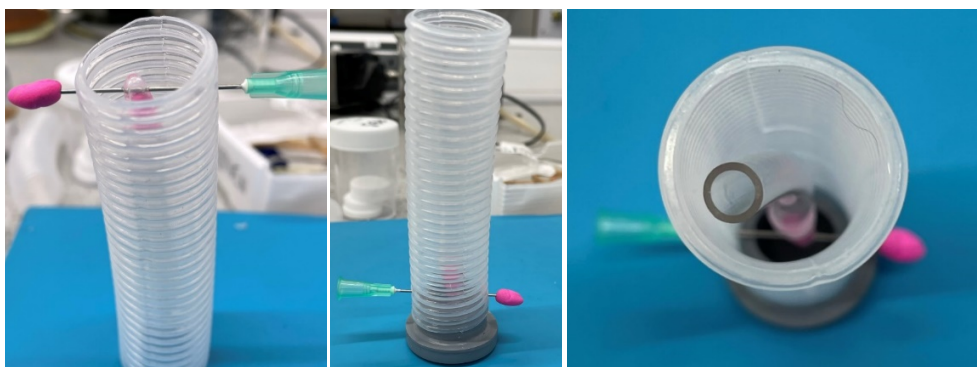
Figure 4.9: Moulds used to produce silicone moulds for hollow cylindrical hydrogels with solid tapered ends.
