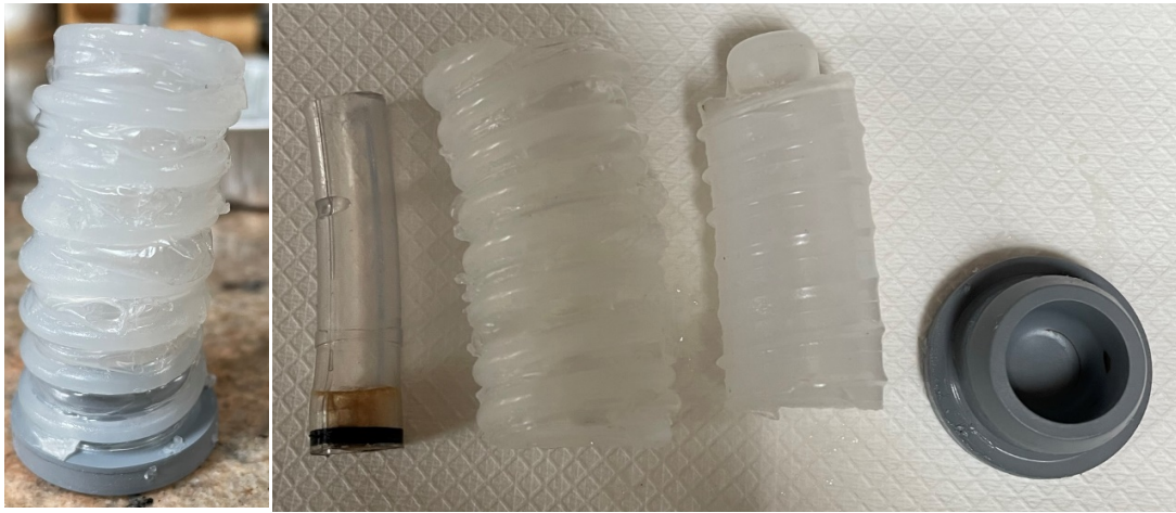
Figure 7.12: Plastic mould containing silicone and the individual components of the mould alongside the silicone mould.
