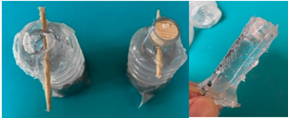
Figure 7.10: Attempt at making silicone moulds for hydrogels from building sealant silicone.
