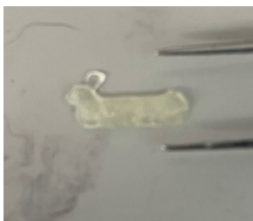
Figure 4.24: Partial formation of the hydrogel half-sized rod cured during the fourth sample print.
