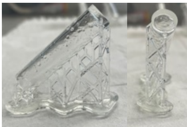
Figure 7.6: 3D printed moulds with thinner walls. The supports and the base of the supports were removed from the mould and IPA washing took place.
