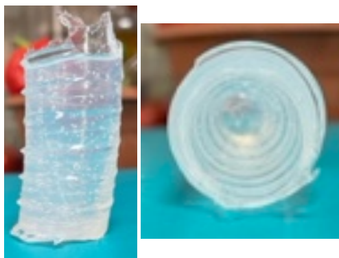
Figure 4.35: Solid silicone removed from its mould.
