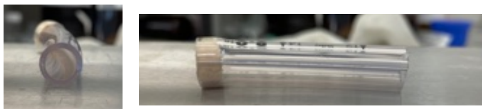
Figure 4.6: Pliable moulds made to produce rods with an 8mm diameter and lengths between 40-46mm.
