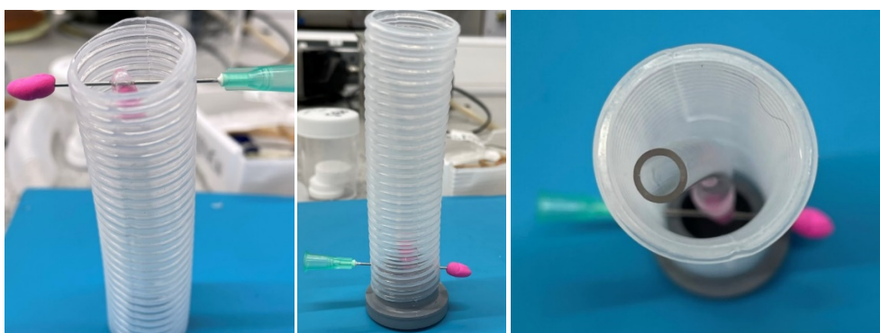
Figure 7.16: Moulds used to produce silicone moulds for hollow cylindrical hydrogels with solid tapered ends.
