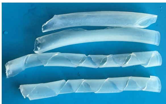
Figure 4.46: Image of the quincke end, blunt end and helical hydrogels post-swelling.
