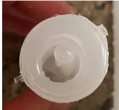
Figure 4.40: Silicone mould successfully created to produce a hollow hydrogel with thinner walls.
