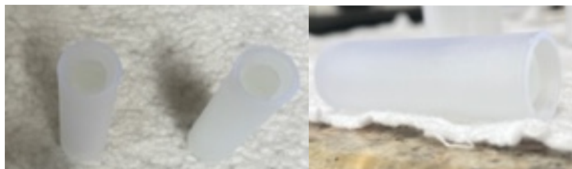
Figure 7.8: 3D printed moulds that were produced to make the silicone moulds for the hydrogels more accurate.
