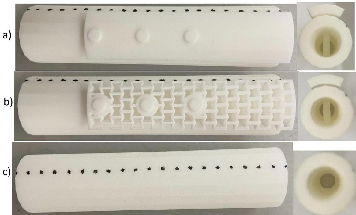
Figure 5-9: Printed parts showing the black markers at which the strain was calculated. A) is the case with a conventional plate, b) is the case with a stiffness graded auxetic plate and b) shows the case with just a bone.
