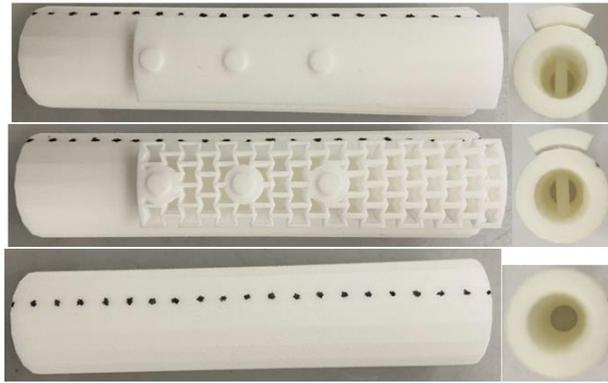
Figure 5-23: Samples used for the compression tests. Sample with a conventional plate (top), sample with an auxetic graded plate (middle), and sample without a plate (bottom).
