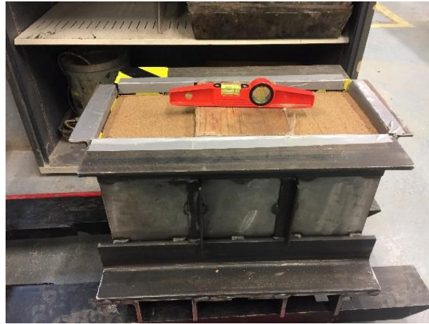
Figure 8.4 Test specimen after compaction
