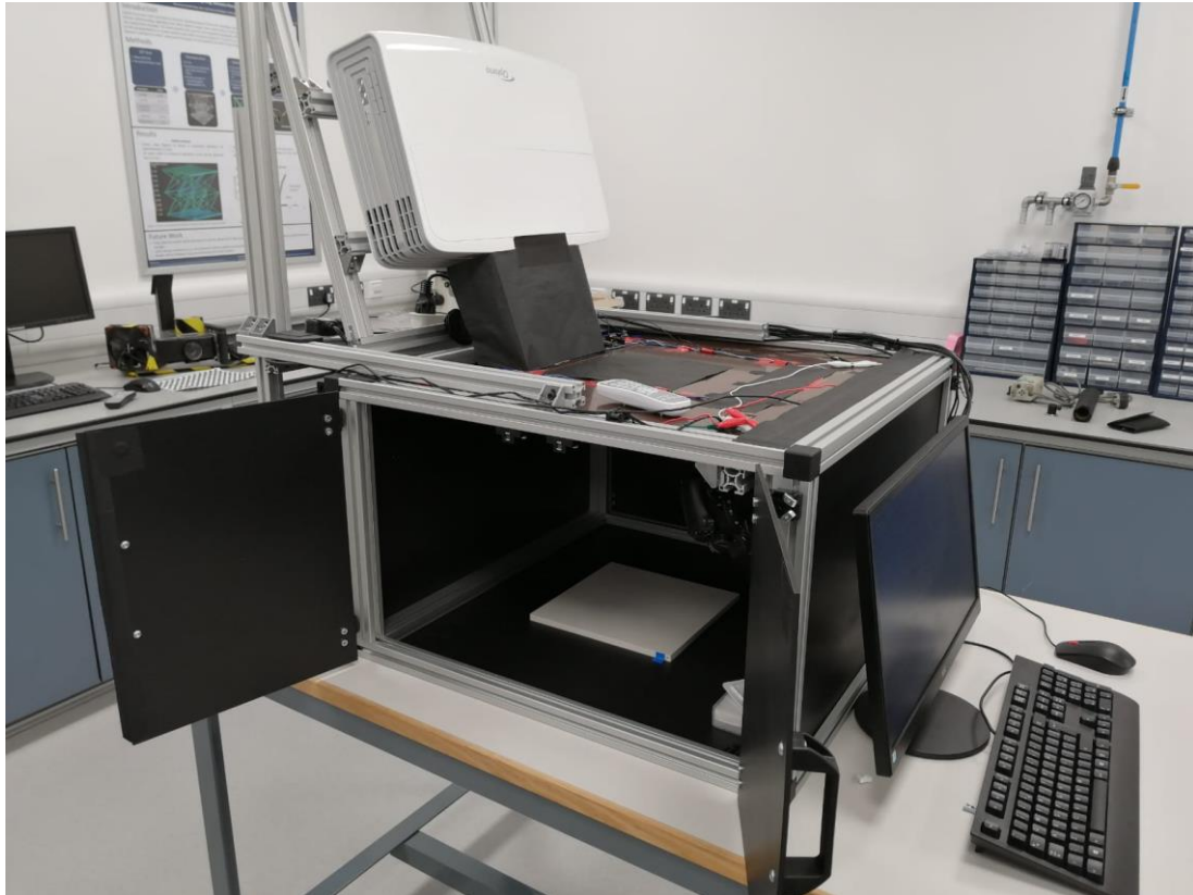
Figure 3.2.c. Initial prototype of the multi-view FP system used for initial testing.
