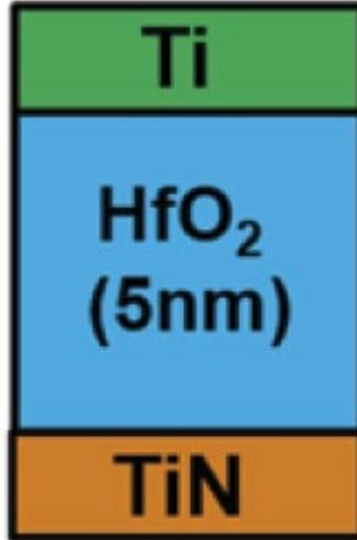
Fig. 2-21. Three-layer ReRAM. HfO<sub>2</sub> is the TMO layer, Ti and TiN are the electrodes [72].
