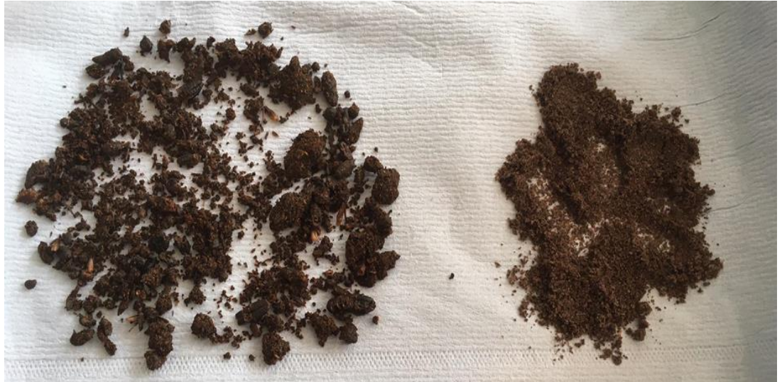
Figure 32: Failure to adequately mill BLOD using the cutting mill - Left: Oven-Dried, unable to be completely milled using the cutting mill. Right: Drum Dried Powder for comparison
