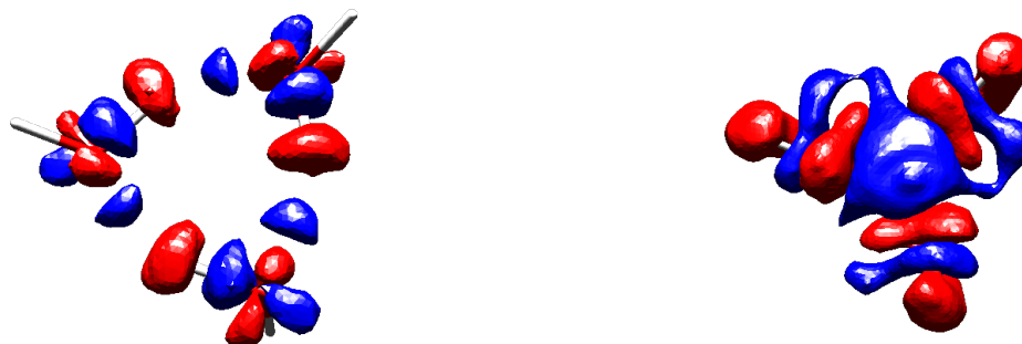
Figure 4.3: The difference in the electron density between the full system and its isolated monomers, of the TPSS-EFM optimised water trimer at |\mathbf{B}| = 0.1 a.u. (left). The electron density at the |\mathbf{B}| = 0 a.u. equilibrium geometry (right).
