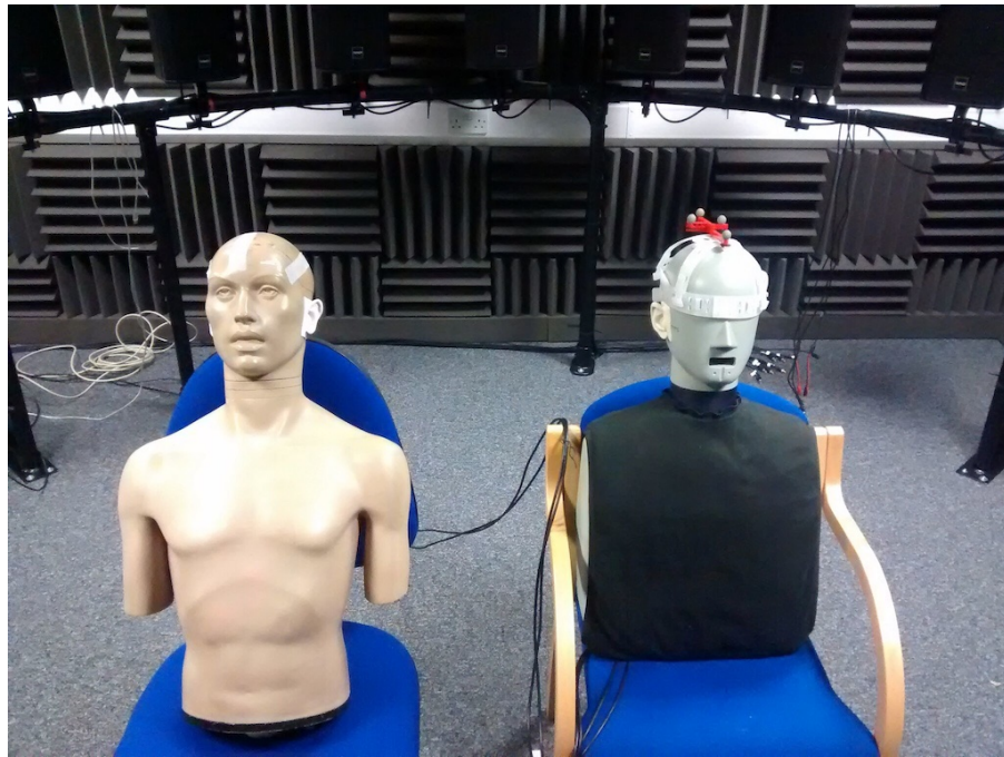
Figure 3.4: HATS (with motion-tracking crown) and KEMAR inside test room in Glasgow.
