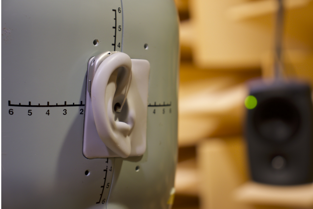
Figure 5.33: HATS wearing the Oticon Open-S 1 Mini RITE.
