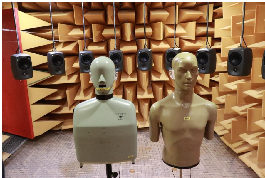
Figure 3.5: HATS and KEMAR inside anechoic test room at Eriksholm.
