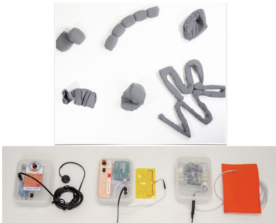
Figure 75. Soft shapes, sensors, and actuators making part of the Soma Bits kit.
