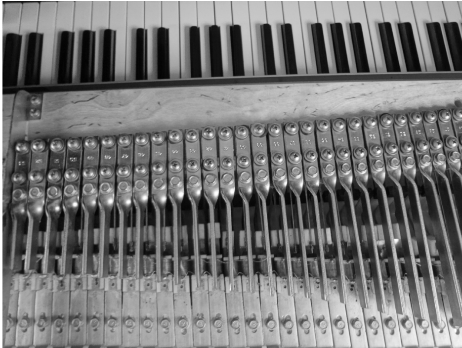
Figure 92. Fender Rhodes electric piano tine-based sound generating mechanism.
