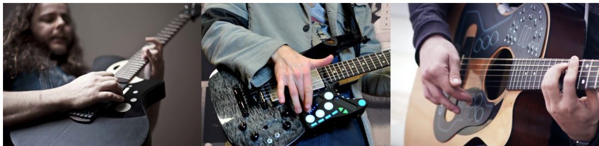
Figure 43. The Sensus Guitar, the Guitar Wing and the ACPAD's in-instrument touch inputs.
