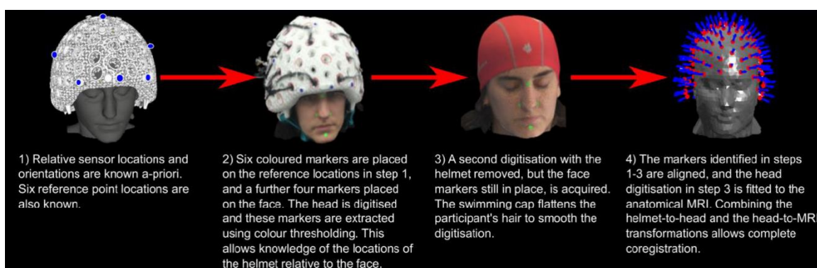
Figure 2.13 – Co-registration pipeline. Sensor locations within the helmet are known from the design process. 3D digitisations of the participant's head with and without the helmet are obtained and co-registered to an anatomical MRI to determine OPM positions and orientations relative to the brain. (Adapted from Hill et al., 2020).
