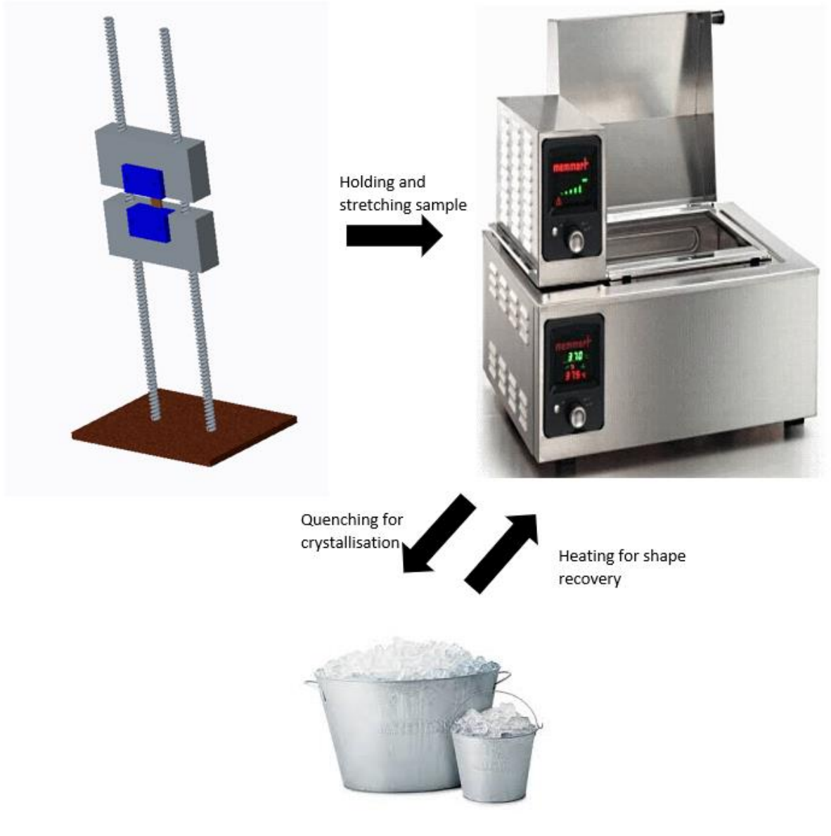
Figure 3.4: The equipment of shape memory experiment (water bath machine for heating process while ice water for quenching process)
