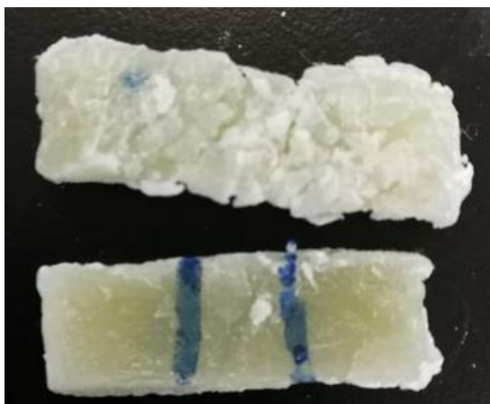
Figure 4.2: Crystal palmitic acid formed on the surface of NRL specimen (swelling duration >120 minutes)
