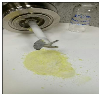
Figure 3.28. The pre-synthesised batch of PMMA-CTA ( M_n = 15,000 g/mol). This was added to the autoclave and redispersed before addition of 4VP.
