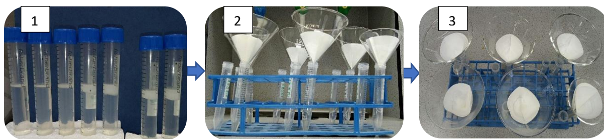
Figure 4.10. Procedure to determine the crosslinking density of PMMA- b -P4VP that was crosslinked by DVB. Dissolution of material in chloroform (1), Sample filtration (2) and soluble (in the tube) and insoluble (on the filter paper) components (3).
