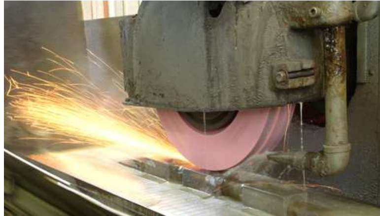
Figure 1: From [1]. Image taken during the surface grinding of a workpiece. Sparks can be seen being emitted from the cutting occurring in the grinding zone. The nozzle in the bottom right is closely positioned to the wheel to deliver grinding fluid into the grinding zone.
