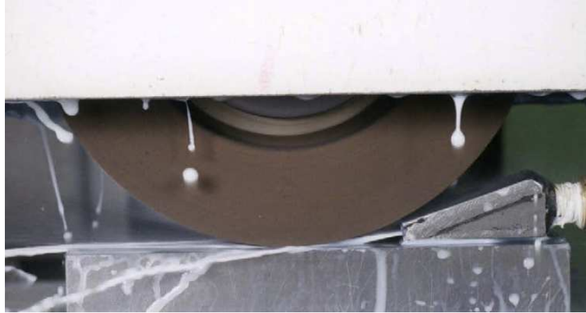
Figure 5: From [60]. Image taken of simulated grinding whereby a thin gap exists between the grinding wheel and workpiece. The grinding fluid is observed to travel through the gap in a far greater amount than it would be expected to travel through the grinding zone.
