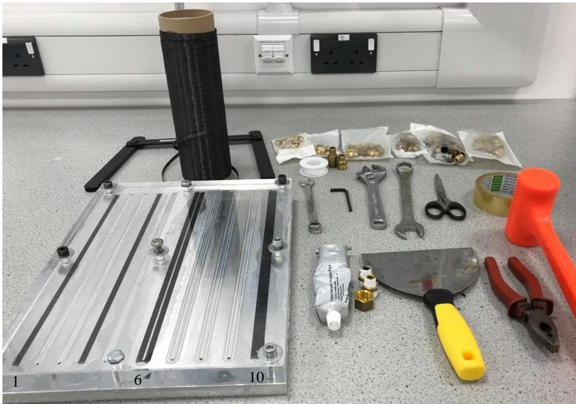
Figure 40 - A 2mm gap can be observed in cavity 6. The cavity 1 is designed to contain single tow (bound) and no gap while cavity 10 is designed for two tows (bounded) and no gaps.
