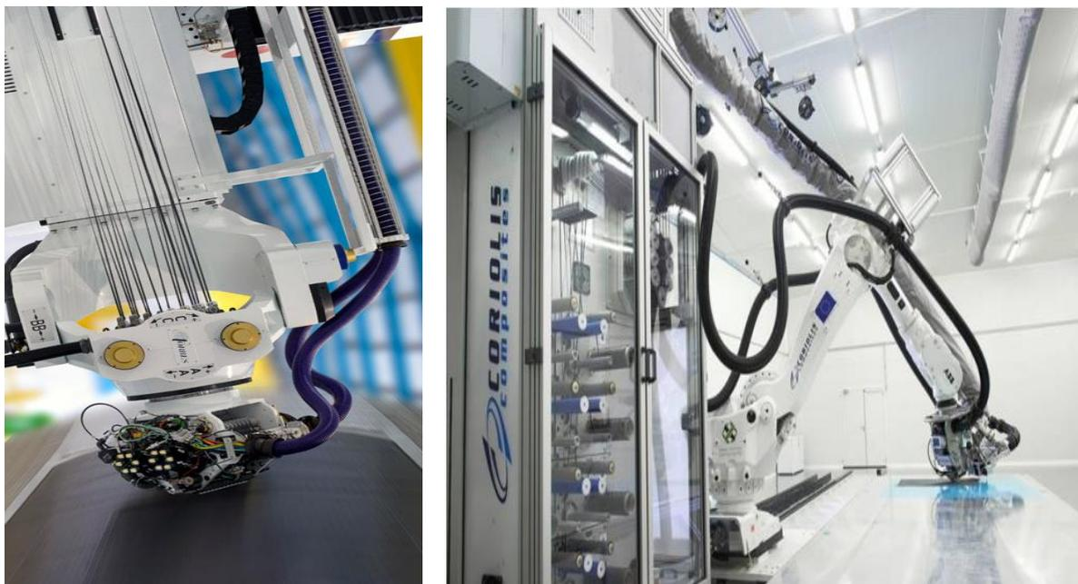
*Figure 7 - Automated Fibre placement Machine – Gantry M-Torres fibre layup (left), Coriolis Robot Arm (right)*
