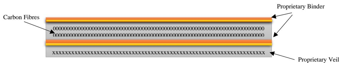
Figure 8- PRISM TX1100 Dry Tape schematic
