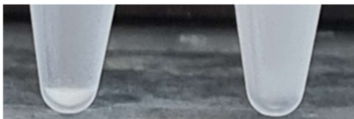
Fig. 6.2: Digital images of the two follow-up tests with 2-methyl-1-propanol. (Left) 50 \mu\text{L} of BSA solution added to 1 mL solvent and mixed for 1 minute. (Right) 247.5 \mu\text{L} BSA solution added to 1 mL solvent and mixed for 2 minutes.
