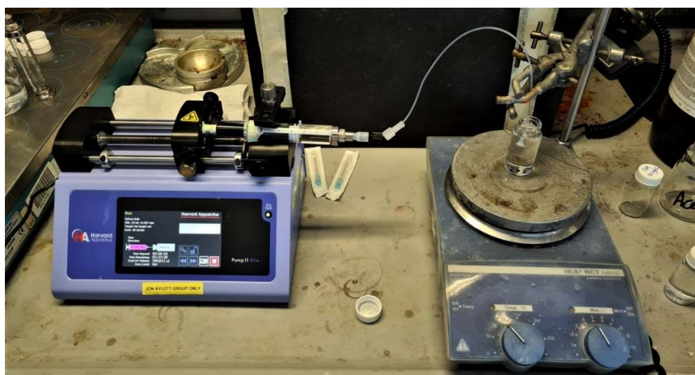
Fig. 2.5: Experimental setup for the single flow continuous production method. Aqueous protein solution was pumped through a single piece of FEP tubing directly into the stirred solvent reservoir.
