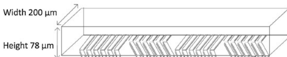
Fig 1.8: A schematic of a staggered herringbone mixer chamber showing the asymmetric herringbone ridges. Adapted from [135].
