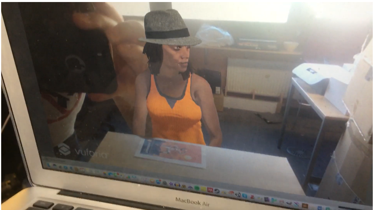
Figure 5.3.) View of a virtual character, attached to a Vuforia marker, being positioned in relation to an invisible occlusion material, itself positioned where a real-world table would be placed. This creates the illusion of a virtual character sitting behind, and being hidden by, a real-world object. Due to the use of a virtual table made out of occlusion material, and the lining up of this table with the real-world table, the camera can be moved and the illusion of the character sitting behind the table is maintained from any angle
