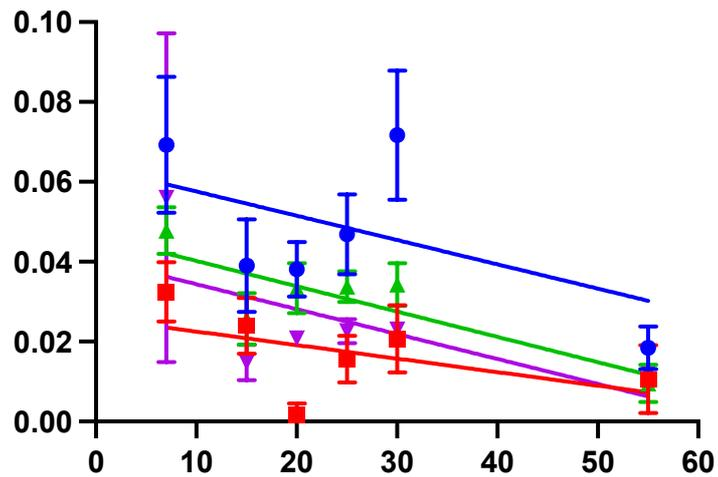
Figure IV-11: Effectiveness of line cleaning solution at a range of temperatures between 7.5°C and 55°C (n=6, ± SD). The impact of increased temperatures was assessed in four beer styles SL3 (blue), ST1 (red), PKA1 (green), and SC1 (purple). Increased line cleaning temperature did not have an impact between 7.5°C to 30°C. At 55°C microorganism recovery is significantly reduced ( $p < 0.05$ ).
