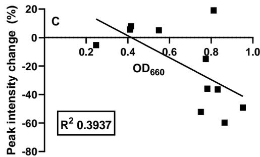
Figure V-9: Optical density (660nm) of forced samples of 96 hrs were plotted versus the relative intensity percentages of each organic acid after the same period. (A) pyruvic acid, (B) citric acid, (C) malic acid
