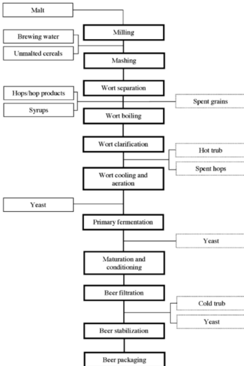
Figure I.1: Schematic of the brewing process, sourced from Willaert (2007b)
