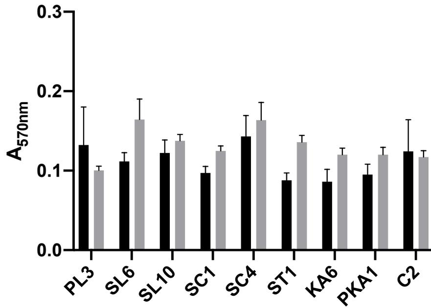
Figure IV-8: Biofilm formation was quantified with two materials, (■) polyvinyl chloride (PVC) and (■) polystyrene (PS) (n=3, ± SD).
