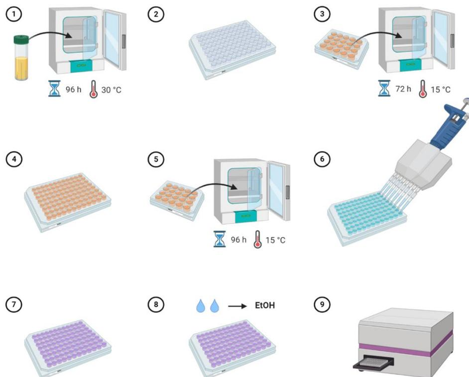
Figure IV-1: Method for quantification of biofilm formation for microorganisms from draught beer. Figure created with BioRender.com (<https://www.biorender.com/>).
