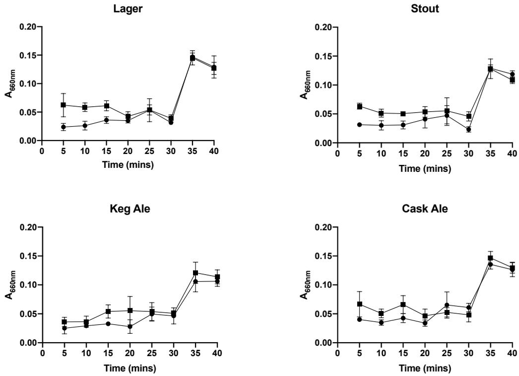
Figure IV-10: Effectiveness of line cleaning versus established biofilms 5 – 40 minutes ( $n=3$ ,  $\pm$  SD) with washing once ( $\bullet$ ) or twice ( $\blacksquare$ ) post cleaning. Total regrowth of planktonic and sessile microflora ( $A_{660}$ ) was quantified as a measure of line cleaner efficacy.
