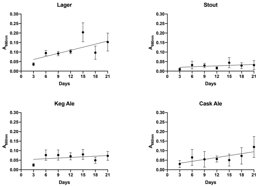
Figure IV-9: Regrowth of biofilm after 30 minutes line cleaning was quantified every 3 days, with replenishment, over 21-day period ( $n=3, \pm SD$ ). Total regrowth of planktonic and sessile microflora ( $A_{660}$ ) was quantified as a measure of line cleaner efficacy.
