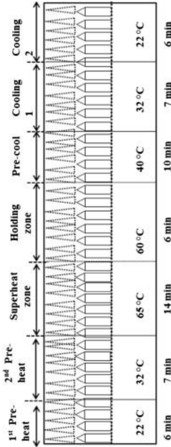
Figure I.2: Schematic of tunnel of pasteurisation, sourced from (Bhuvanewari and Anandharamakrishnan, 2014)
