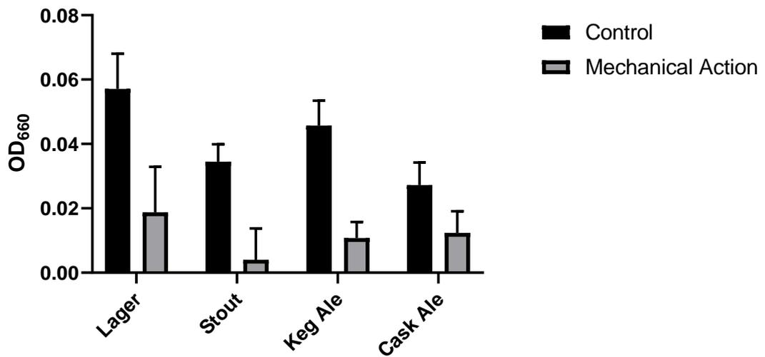
Figure IV-12: Impact of introducing mechanical action into line cleaning. For each sample there is a significant reduction in microorganism recovery versus a static control after a 7-day post-line clean incubation period ( $p > 0.05$ ) ( $n = 6$ ,  $\pm$  SD)
