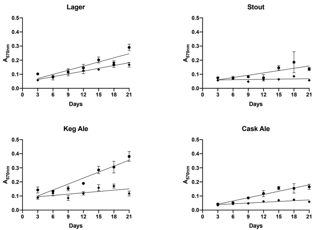
Figure IV-4: Impact of nutrient replenishment on biofilm formation in lager (PL3), stout (ST1), keg ale (PKA1) and cask ale (SC1) where (■) control and (●) replenished.
