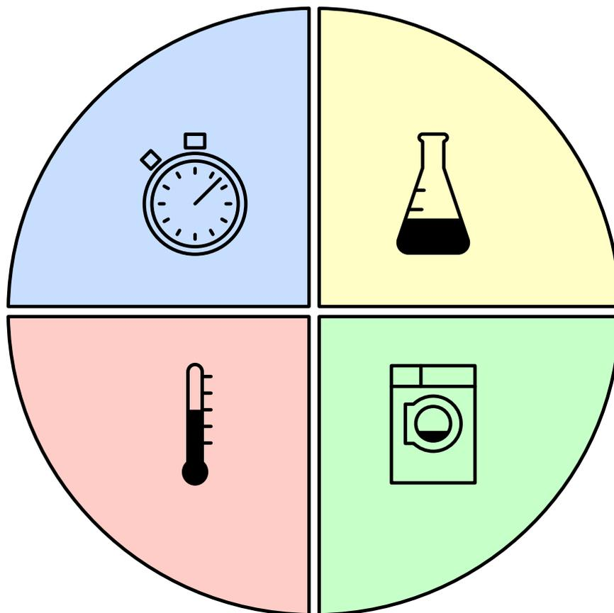
Figure I.3: The four key elements of the 'Sinner circle' - from top left, clockwise; time, chemical action, mechanical actions, and temperature.
