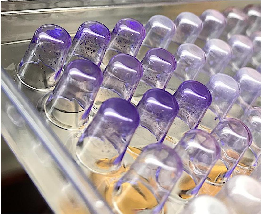
Figure IV-2: Crystal violet stained biofilms in microplate wells. In triplicate from (top to bottom) in lager (PL3), stout (ST1), keg ale (PKA1) and cask ale (SC1).
