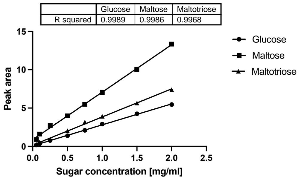
Figure V-2: Standard curve of glucose, maltose, and maltotriose (n=3)
