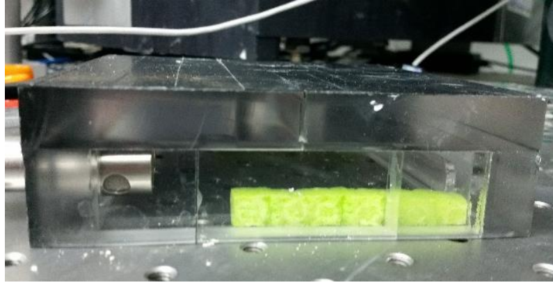
Figure 26: The custom-built covers used throughout this manuscript. The green strip is a sponge that was wet to boost the internal humidity. These covers were also wrapped in black tape to control the amount of light within for video capture.
