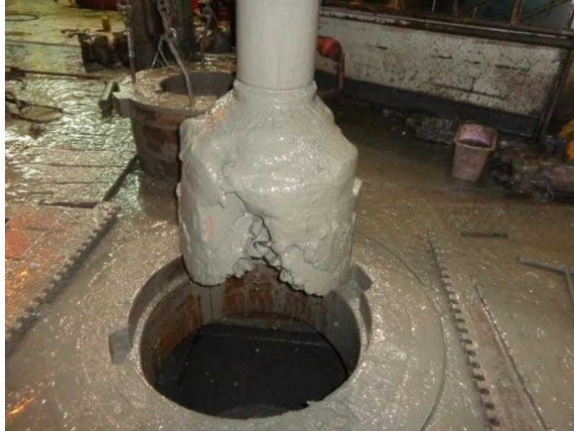
Figure 18: A drill assembly that has been brought back to the surface. As soil and clay becomes adhered to surface it reduces the effectiveness of the drill until it can no longer penetrate the surrounding rock
