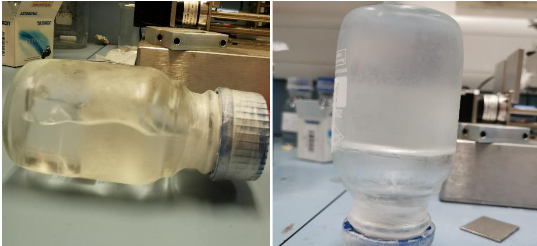
Figure 17: A laponite stock gel that has been perturbed and then left to age. Left image was taken immediately after perturbation while right image was taken 24 hours after perturbation. The left image shows that when initially disturbed the gel can flow much like a liquid, however, when left to stand we observe that the fluid will not flow under the action of gravity alone (right).
