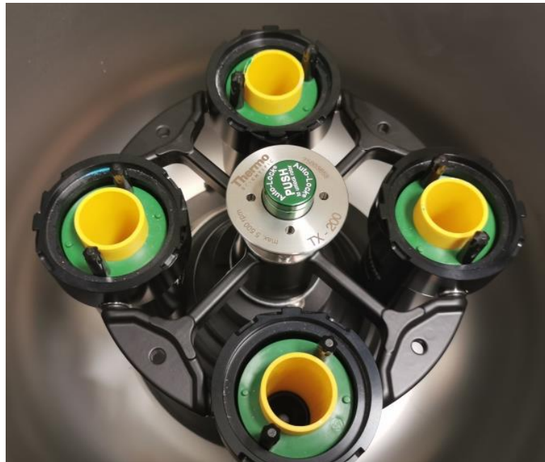
Figure 84: Centrifuge fitted with the swing arm rotor, internal bucket radius is 16.5 cm, total radius 17.5 cm.
