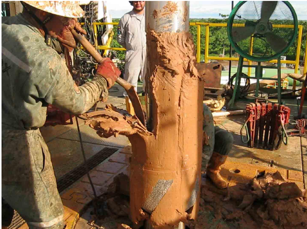
Figure 52: An example of the issue of bit balling. Clay and sediment has adhered to the drill assembly to such a significant degree the operators are using a spade to remove the thick layers built up. Image was taken in Columbia by Schlumberger employees, obtained from [110].
