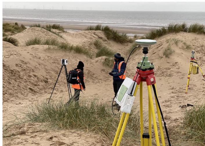
Figure 5.2. GNSS base station and TLS targets set up in the study area.
