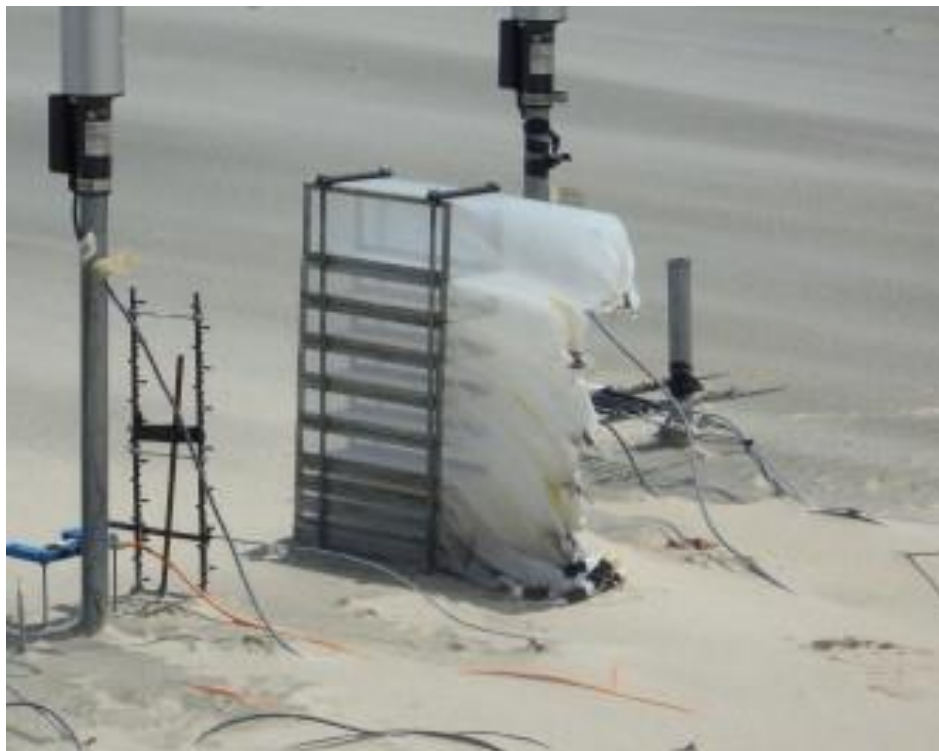
Figure 2.8. A vertical sand trap used for measuring horizontal sand flux.
