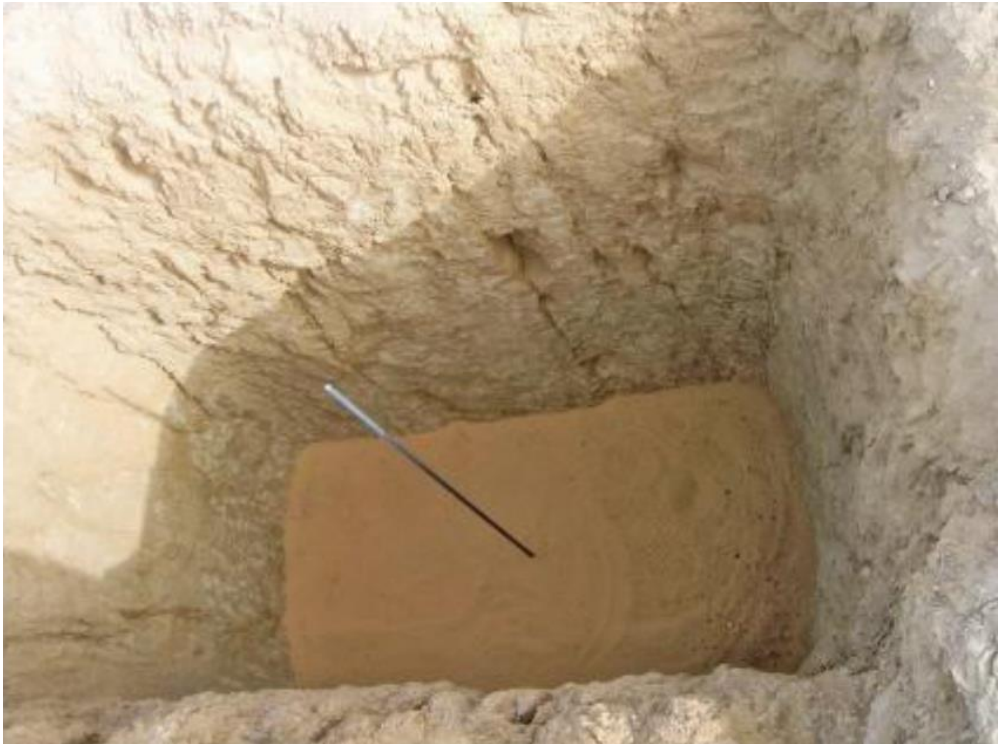
Figure 2.9. Horizontal sand trap used for measuring vertical sand flux.
