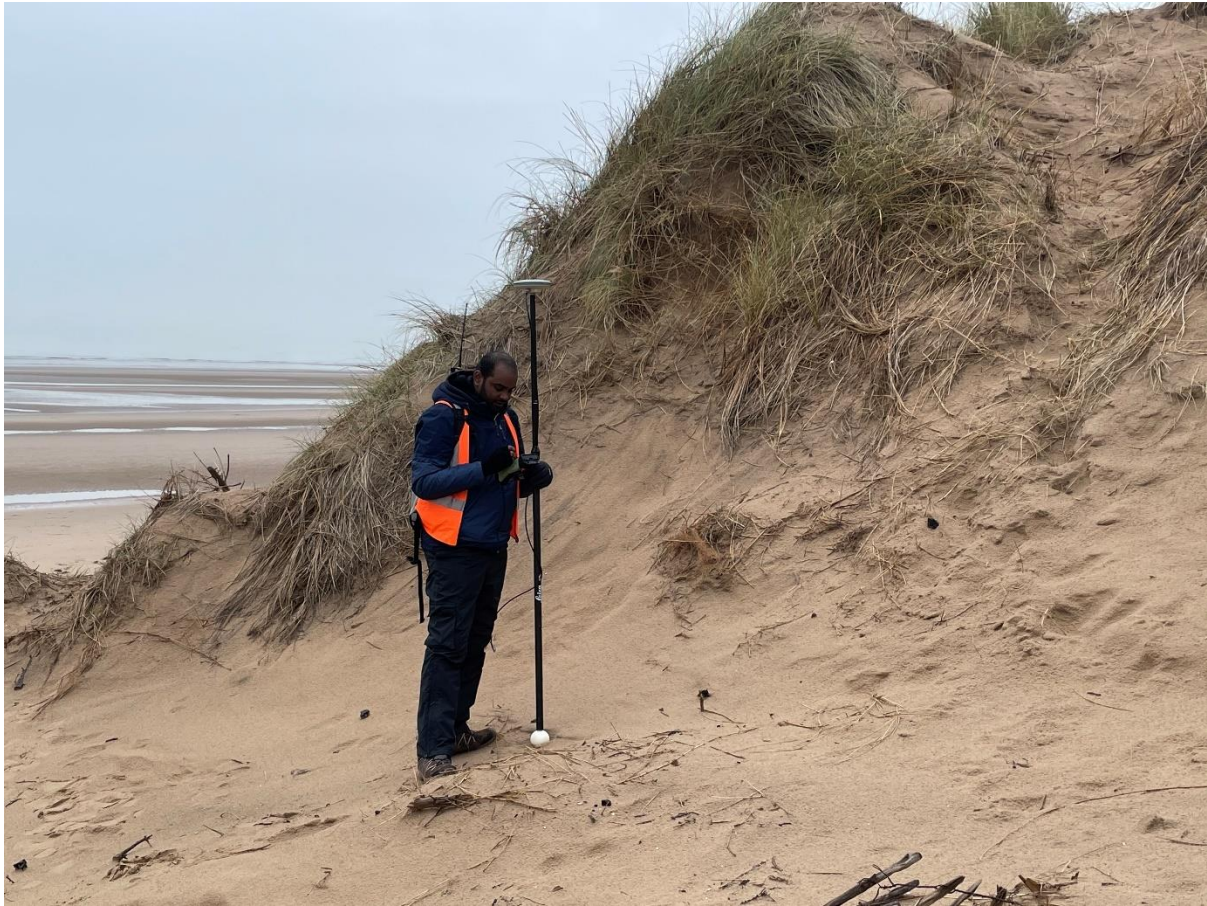
Figure 5.4. Collection of RTK GNSS data on the frontal dunes of the north part of the study area at Formby.
