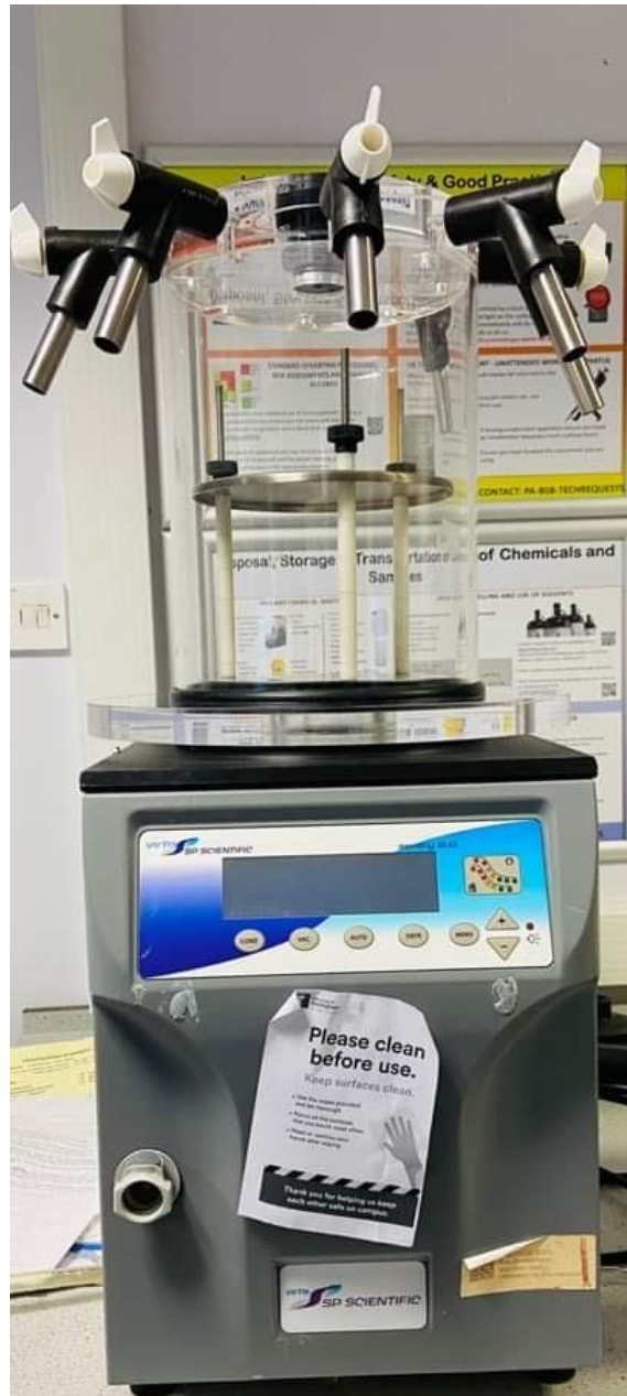
Figure 8 Freeze dryer, Virtis benchtop lyophiliser® (SP scientific sentry 2.0)
