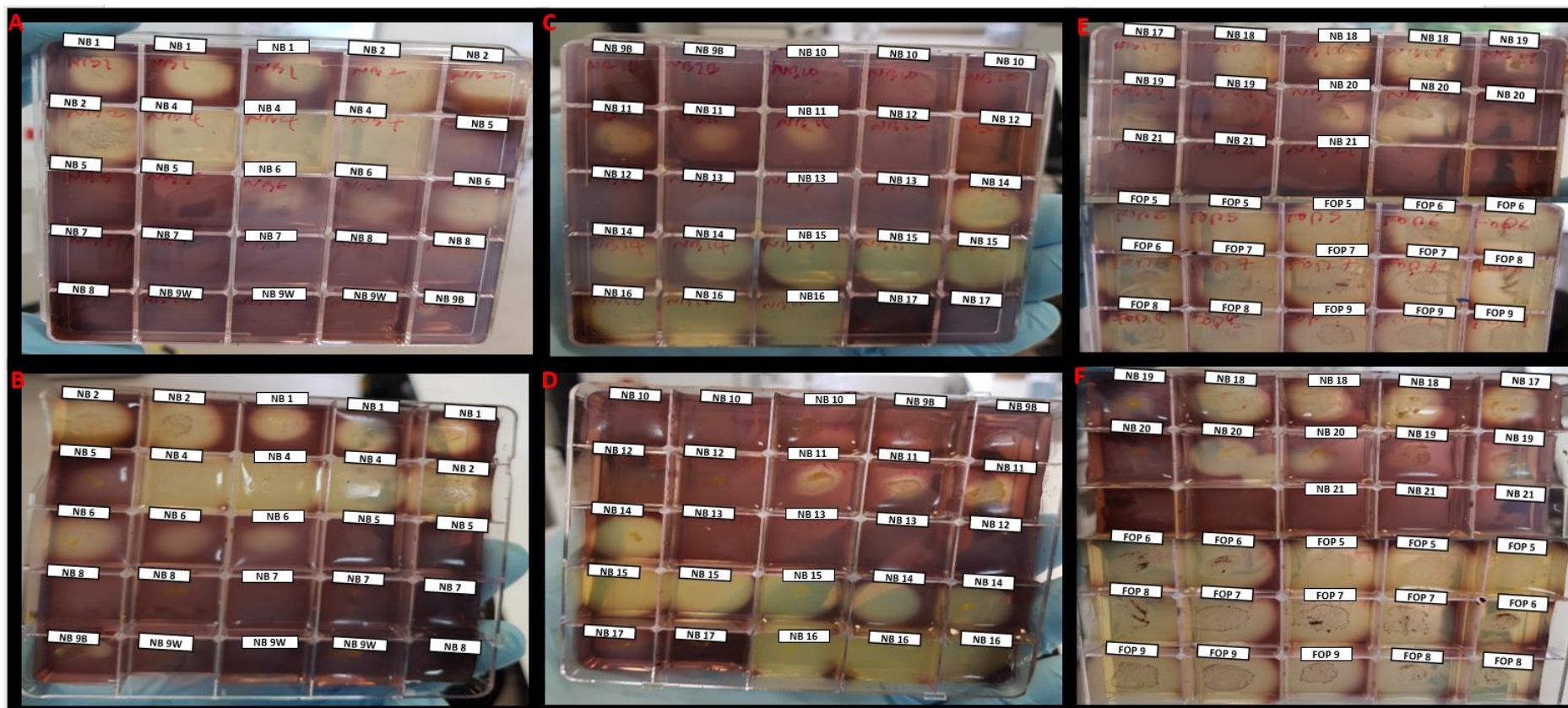
Figure 5. 5: Bioprospecting to produce cellulase by isolates on carboxymethyl cellulase (CMC) agar in multi-well plates. Plates A, C and E are rear views of the multi-well plate, while B, D and F are front views. Positive results were inferred with at least two positive results from the triplicate assays by forming a clearing zone around the isolates. Isolates NB 2, NB 14, NB 15, NB 16, NB 18, NB 19, NB 20, NB 21 and FOP 8 which are marine actinobacteria (chapter two) were the target of this assay.
