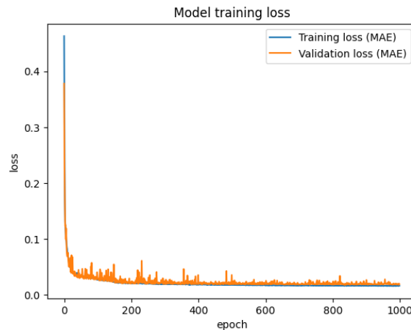
Figure 5.6: The effect of the number of training epochs on training and validation loss.
