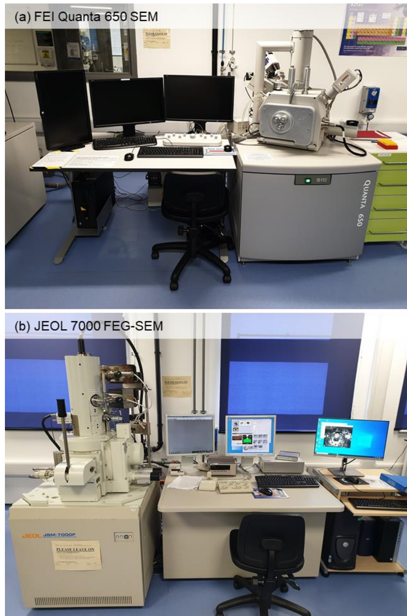
Fig. 3.12. Scanning Electron Microscopes (SEMs) used in this study for imaging. (a) A FEI Quanta 650 SEM was used for imaging in both HV and LV conditions. (b) A JEOL 7000 FEG-SEM was used for superior resolution imaging only in HV conditions.
