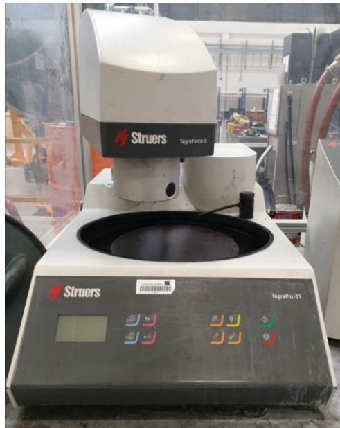
Fig. 3.2. Polishing machine (Tegrapol-21, Struers) used in this research. All samples were ground and polished manually (i.e. without embedding the samples in resin nor using the polishing head).
