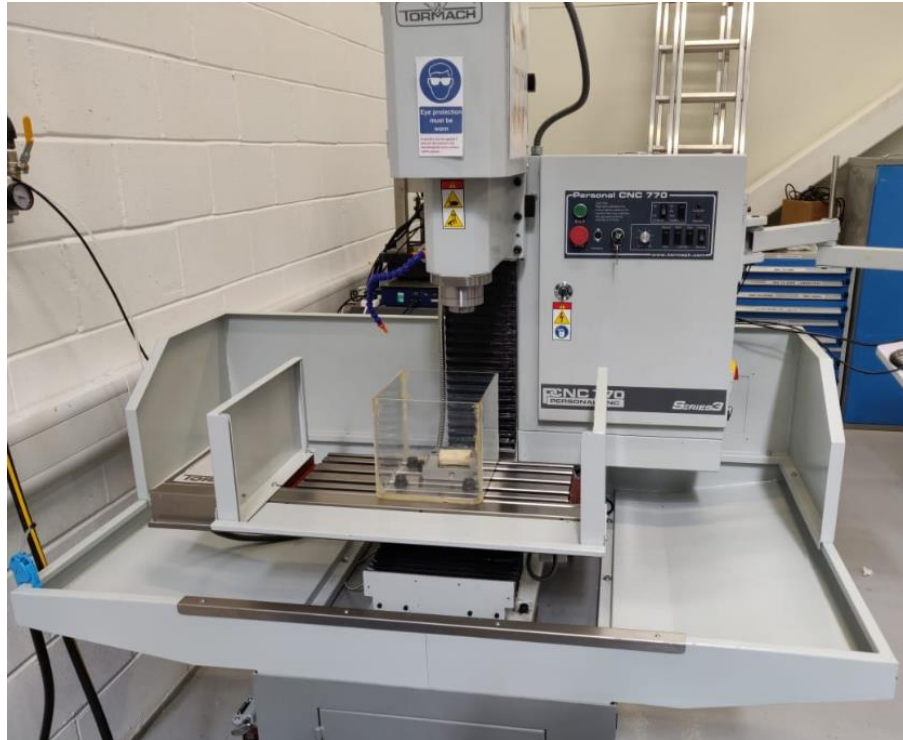
Fig. 3.5. Milling machine (770 PCNC Tormach) used in this study for orthogonal cutting and drilling trials.
