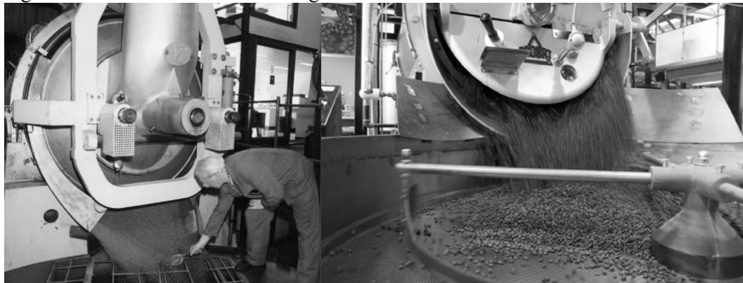
Removal of roasted malt from commercial roasting drum (left), and removal of roasted coffee from commercial roasting drum, showing typical cooling mechanism (right).
