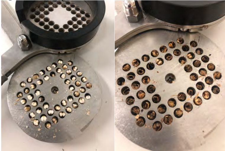
Pale malt (left), and medium crystal malt (right) cut by farinator.
