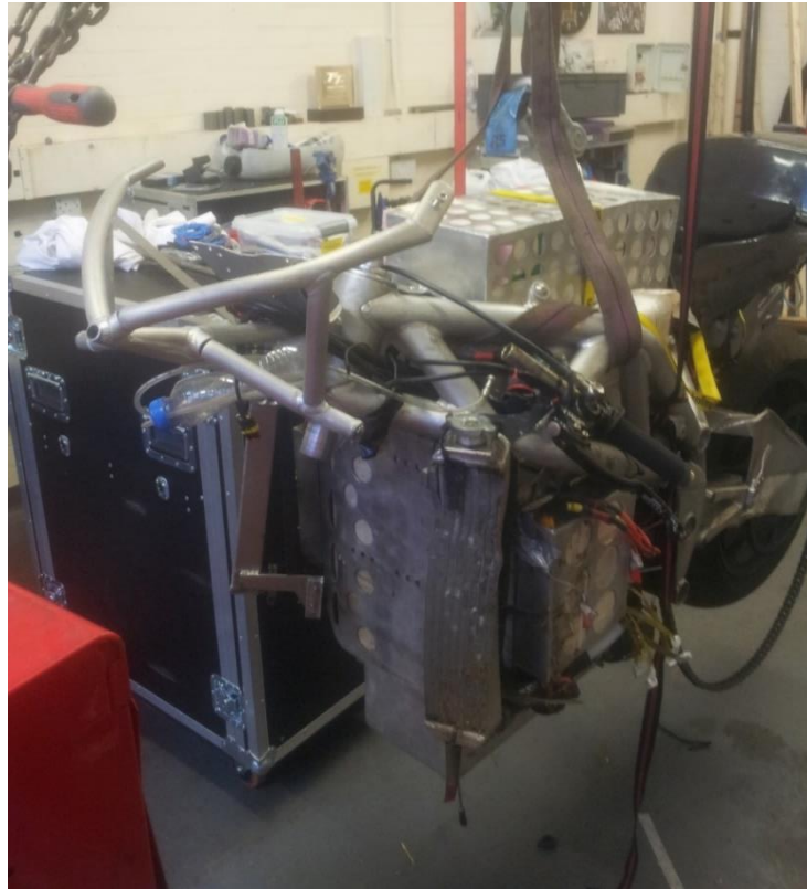
Figure 3.11 - Image of Nottingham motorcycle suspended as part of the measurement process
