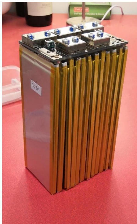
Figure 3.2 - Example battery pack construction.
