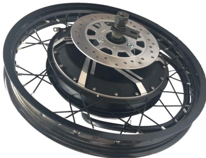
Figure 2.9 - Electric hub motor integration into motorcycle wheel [112]
