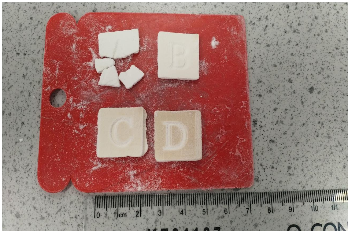
Figure 6.3: Sintering performance of the 50:50 Av/Eu blend in Test 6: Weak layer bonding under laser power of 5W (A); fragile edges and low strength at 6W (B); fragile edges and degradation at 7W (C); degradation and layer misplacement at 8W (D)
