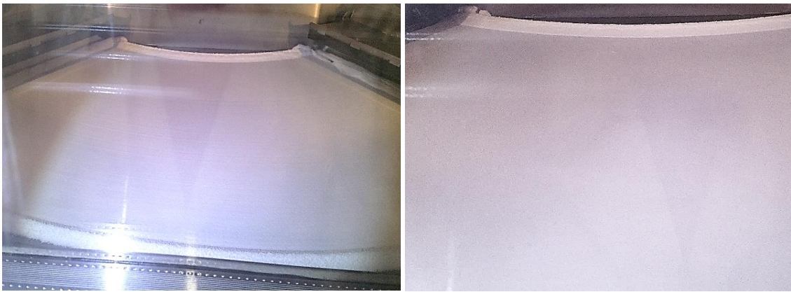
Figure 5.5: Demonstration of improved flow of Foremost 316 powder at 120°C (left) and 150°C (right) by the addition of 2% of Glyceryl Dibehenate
