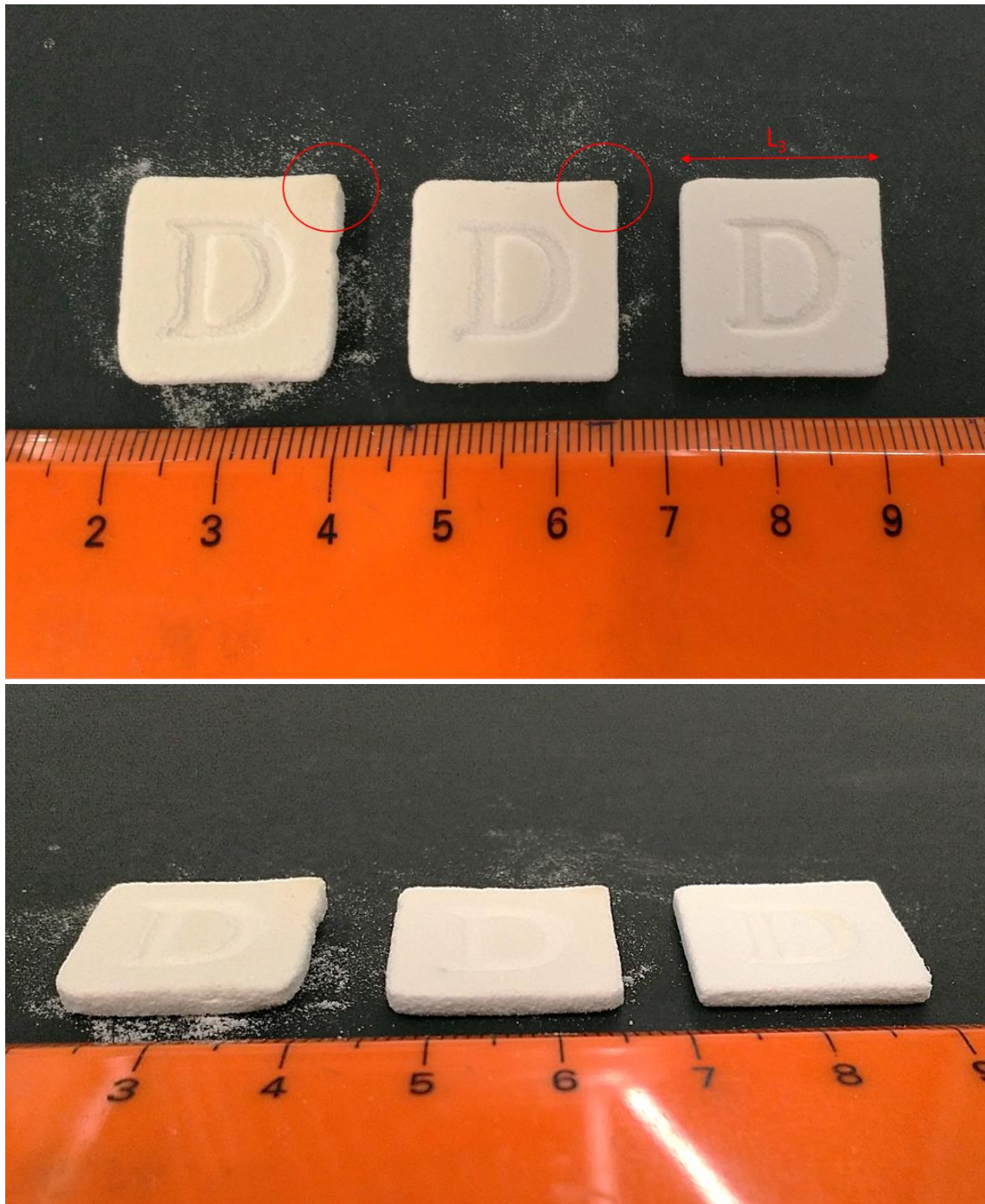
Figure 7.1: General views of the produced parts. Increased dimensional precision from the left 63:37 Av/Eu to the right 37:63 Av/Eu part, as the Eudragit L100-55 increased in the blend. Increased part thickness and degradation from the right to the left, as the ED was gradually increased from 0.0112 J/mm 3 to 0.015 J/mm 3 . The robust top right corners are circled.
