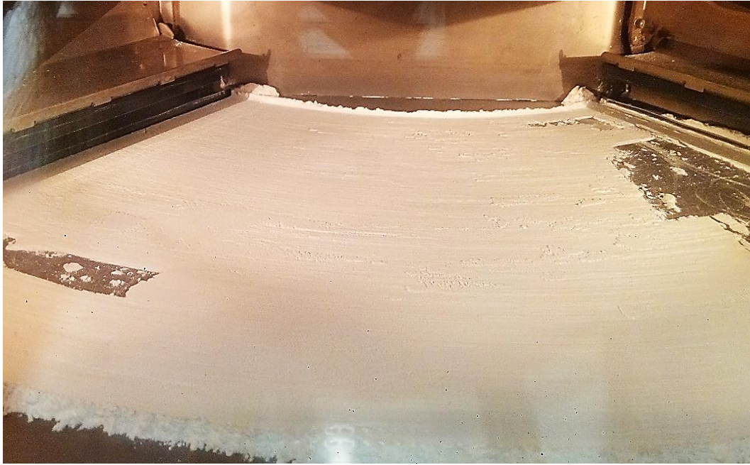
Figure 5.10: Spreading of HPC SSL powder with 1% MgSt at 30°C resulted in high surface roughness
