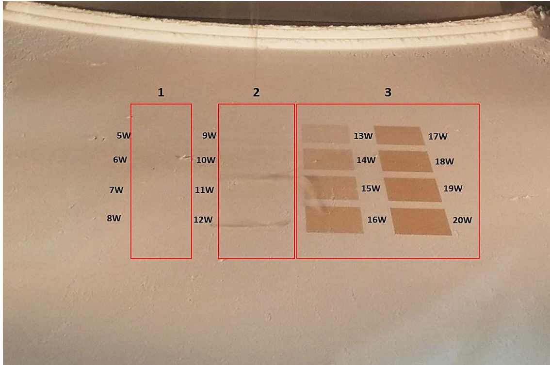
Figure 6.1: Initial trials on the 50:50 Av/Eu blend at various laser powers. Area 1 resulted in poor consolidation; Area 2 resulted in weak layer formation; and Area 3 indicated degradation, whilst the powder fumed
