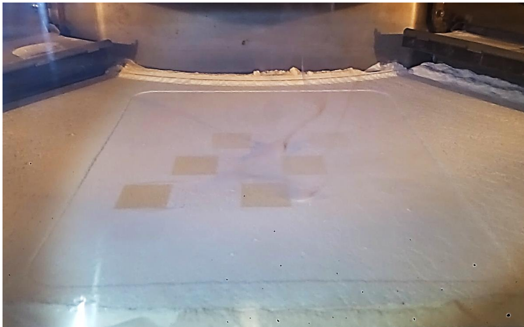
Figure 5.3: Double scanning in Test 6 at low speed resulted in fuming and degradation of Avicel 101
