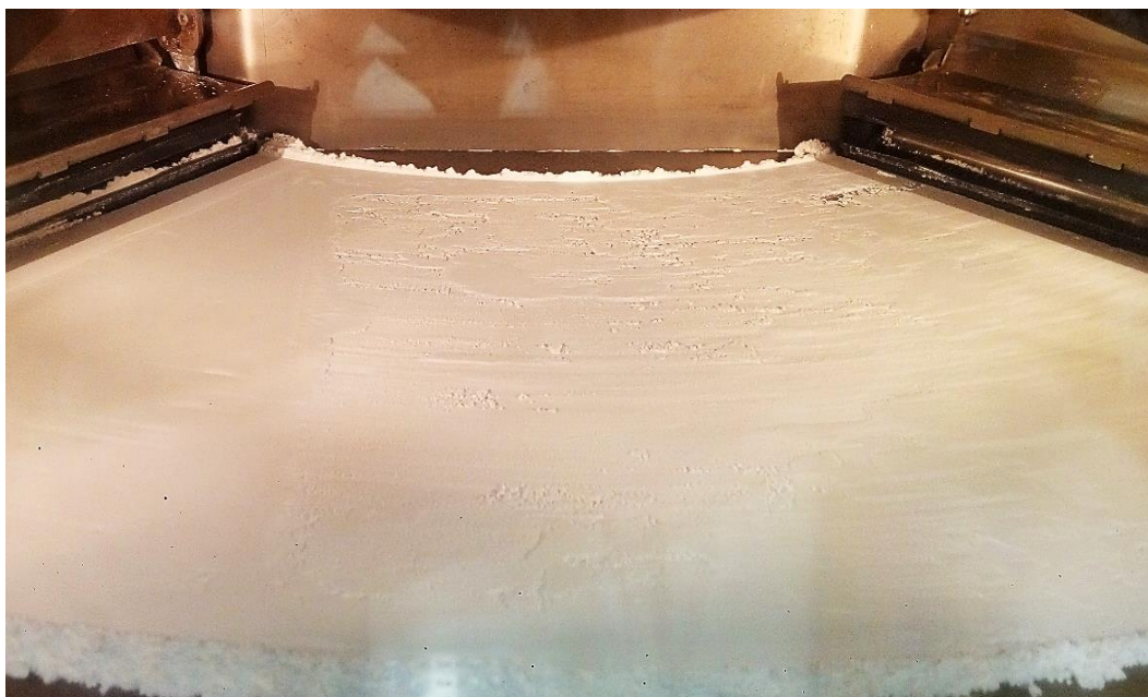
Figure 5.9: Non-uniform spreading of HPC SSL powder at 30°C after the addition of 0.5% MgSt
