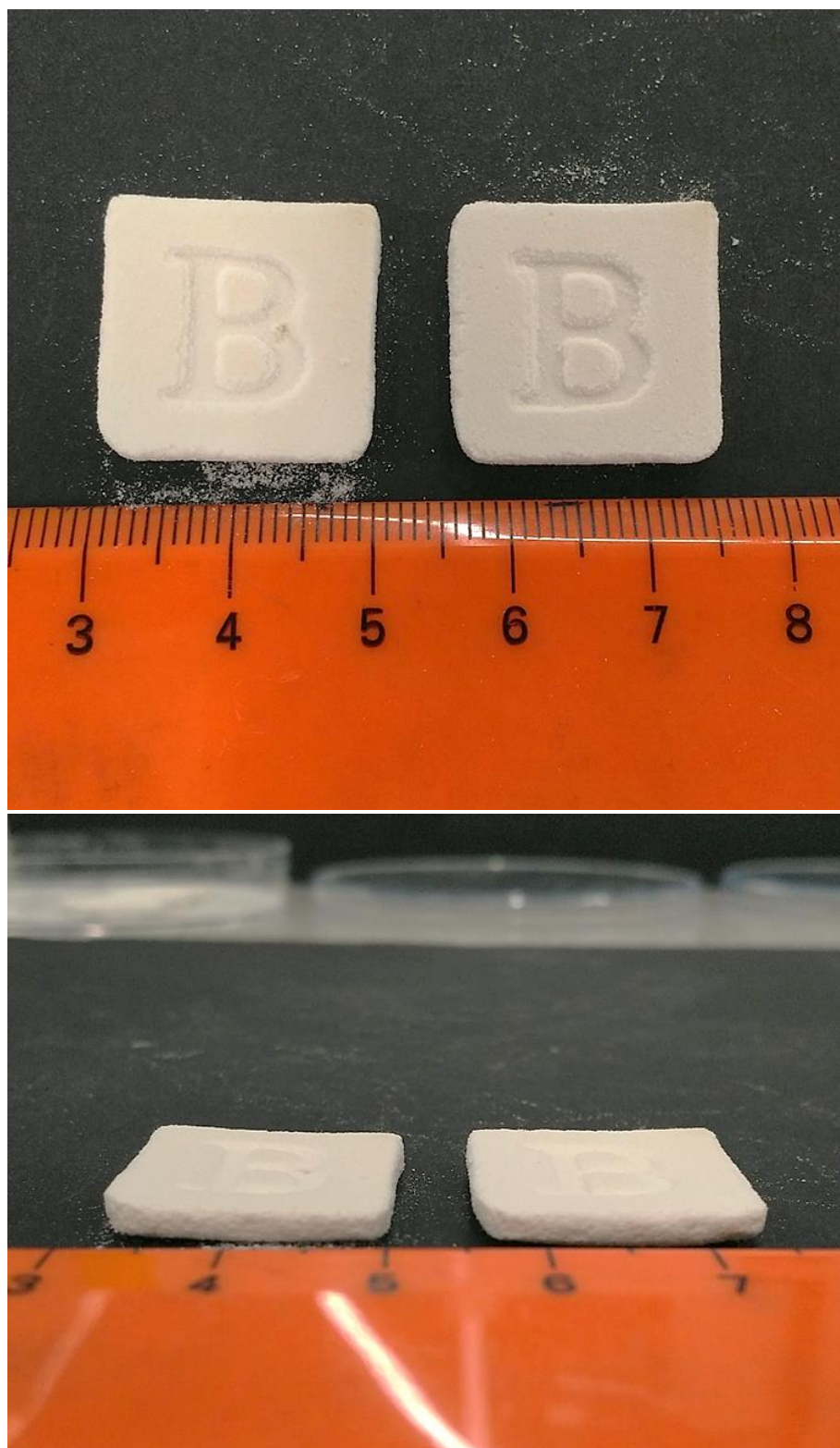
Figure 6.9: Increased precision and clear features for the 50:50 Av/Eu parts produced at ED of 0.0133 \text{ J/mm}^3 ; scanned at 125^\circ\text{C} in the centre top area of the build platform
