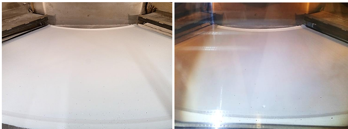
Figure 5.16: Uniform spreading of PolyOx N80 powder at 25°C (left) and 50°C (right)
