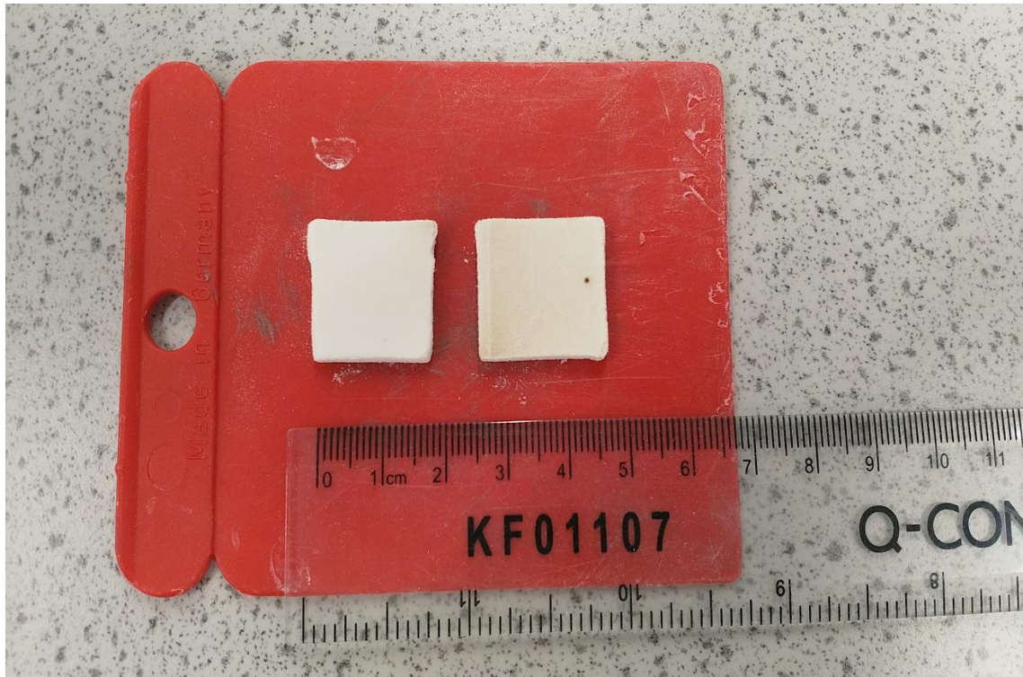
Figure 6.2: Hatching distance at 0.20mm resulted in multilayer formation for the 50:50 Av/Eu blend in Test 5. The yellow colour indicated degradation when scanned at 2000mm/s, while at 2500mm/s the edges were fragile
