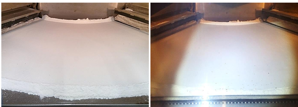
Figure 5.1: Homogeneous spreading of Avicel 101 powder at 25^\circ\text{C} (left) and 170^\circ\text{C} (right)
