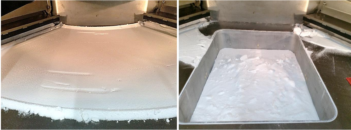
Figure 5.4: Formation of lumps of Foremost 316 powder during spreading at 50°C (left) and 70°C (right)
