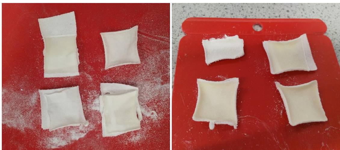
Figure 5.22: Warping and lack of adhesion between layers of PolyOx N80 in Test 11 (left); improved fusion, adhesion and stiffness in Test 12 (right)
