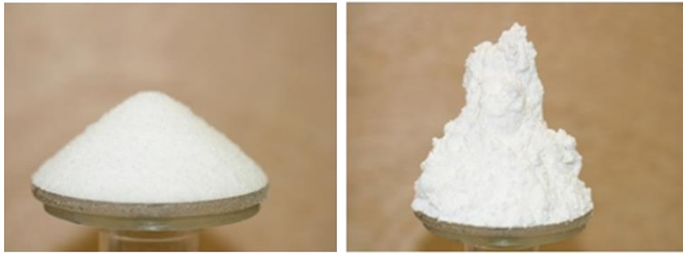
Figure 2.5: Particles of a non-cohesive powder spread evenly and particles of a cohesive powder clump together [85]
