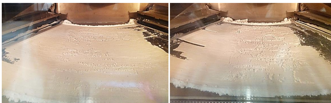
Figure 5.11: Formation of agglomerates and failure to spread HPC SSL with 1% of MgSt added, at 50°C (left) and 75°C (right)
