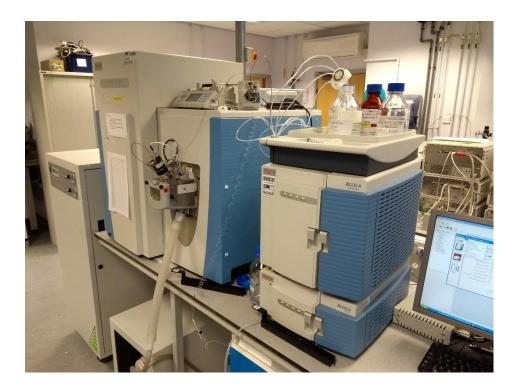
**Figure 2.2:** The LC-MS system set up prior to running samples. Left: Thermo Exactive® mass spectrometer; right: Accela® HPLC.
