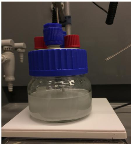
(a) E1:  $\text{SO}_4^{2-}$  and  $\text{HCO}_3^-$  anions present. Cloudy solution is observed at the beginning of the experiment,  $t = 0$ , indicating that the solution is supersaturated.
