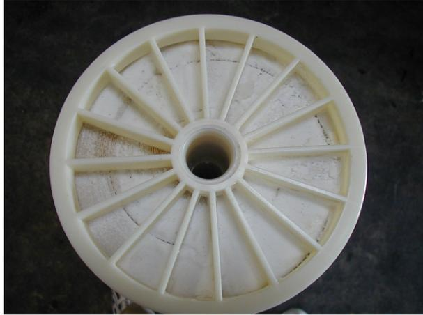
**Figure 1.4:** White  $\text{CaCO}_3$  scale on a spiral wound reverse osmosis membrane module [40].
