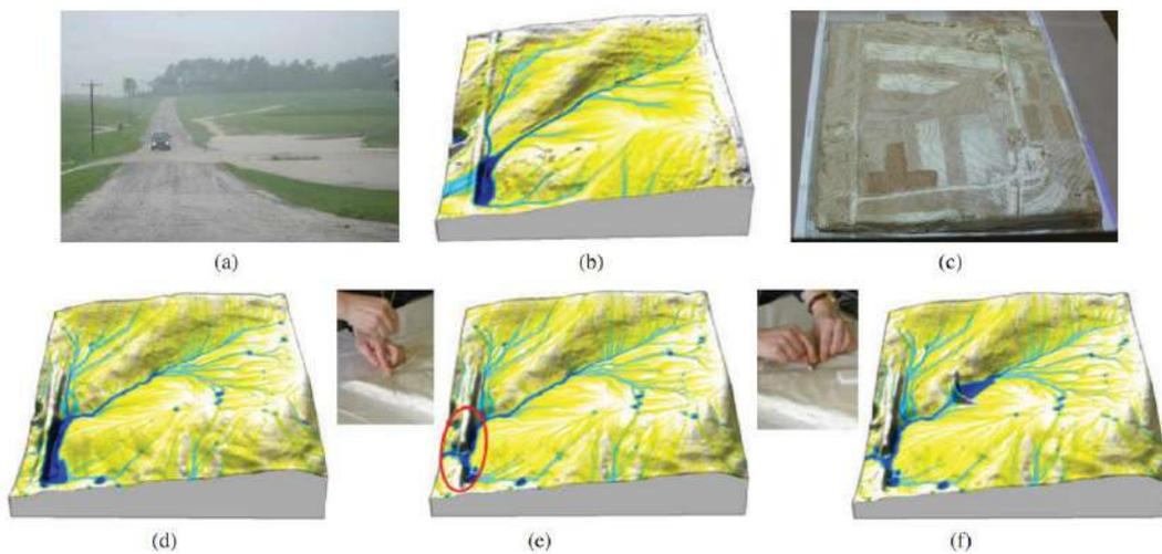
**Figure 2.21.** TanGeoMS modelling of unpaved road (area: 450x450 m<sup>2</sup>) and the simulation of the runoff
