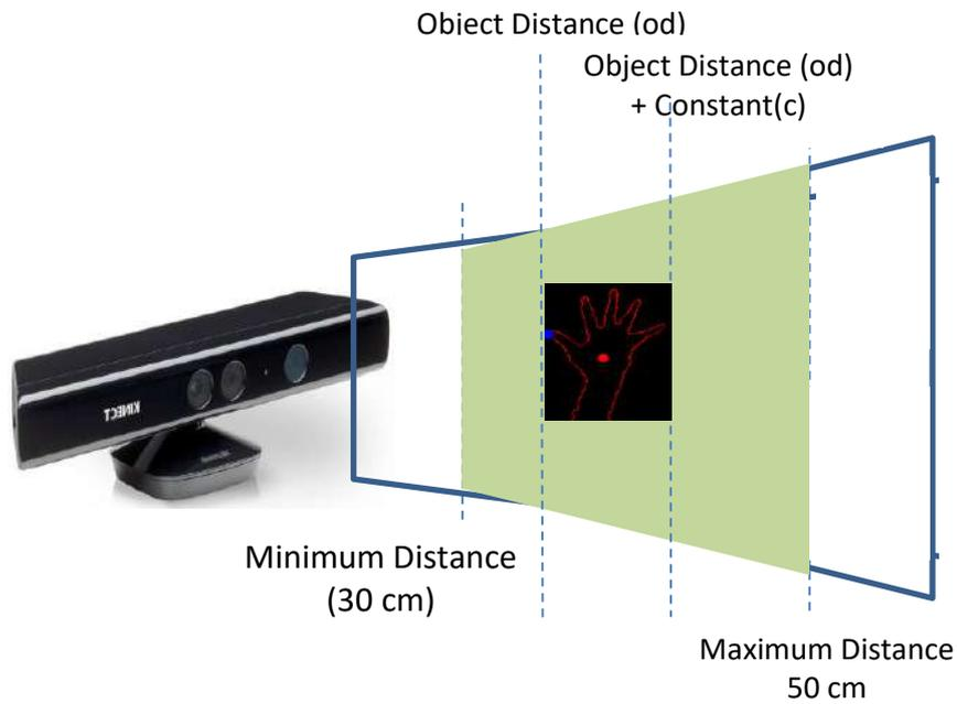
**Figure 5.5.** Range Detection of Kinect
