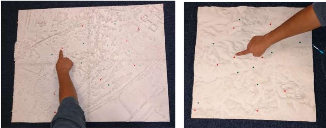
**Figure 5.15.** Finger Kinect Detection on UP Campus Model (left) and Lake District Model (right). Red points represent high surface, green points represent low surface
