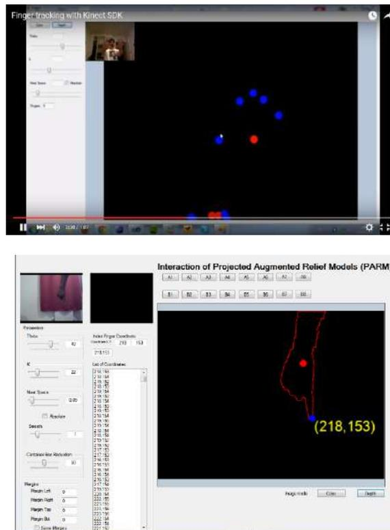
**Figure 5.11.** Finger detection using original Program (top) and Modified program: showing finger's coordinate (bottom)
