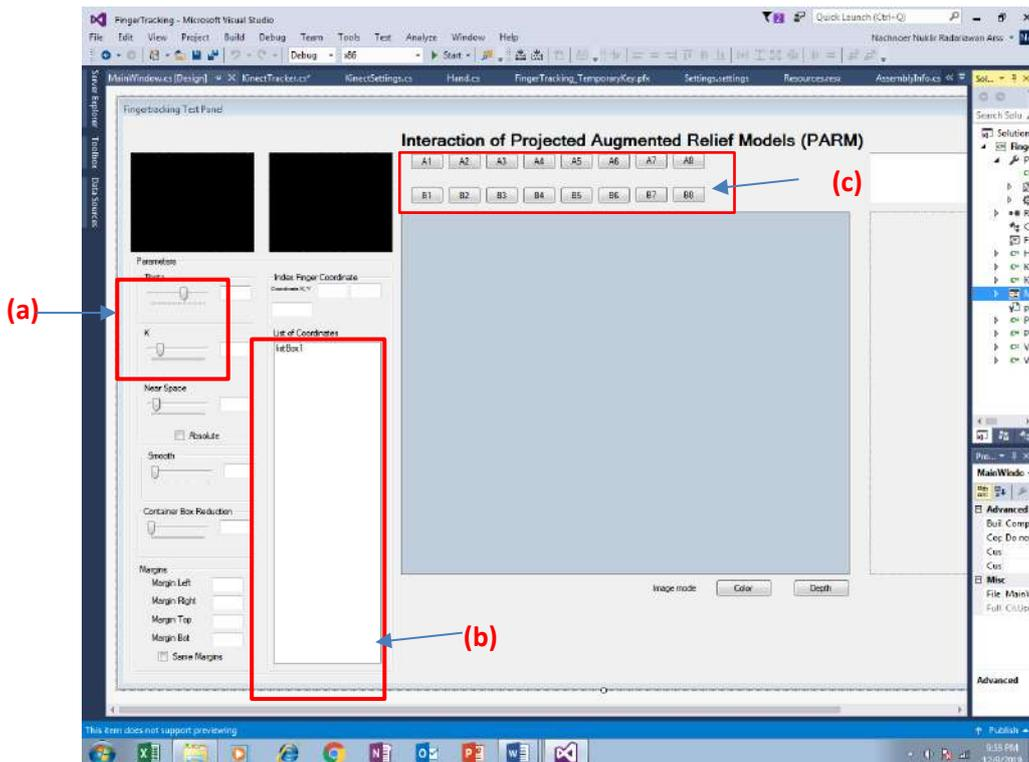
**Figure 5.14.** Modified User Interface of Kinect Program, (a) Theta and K-Value modification; (b) List of detected finger's coordinates; (c) Coordinates capture buttons for point A1-A4 and B1-B4
