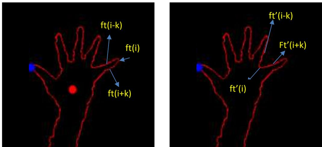
**Figure 5.10.** The k-curvature algorithm (left) and the false-positive result (right)
