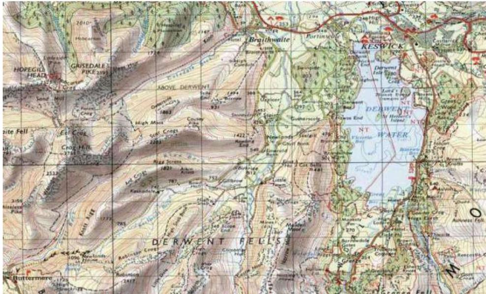
**Figure 2.5.** Hillshading in combination with contours
