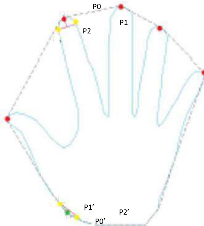
Figure 2.25. Fingertip detection using a 3-point method classifier.
