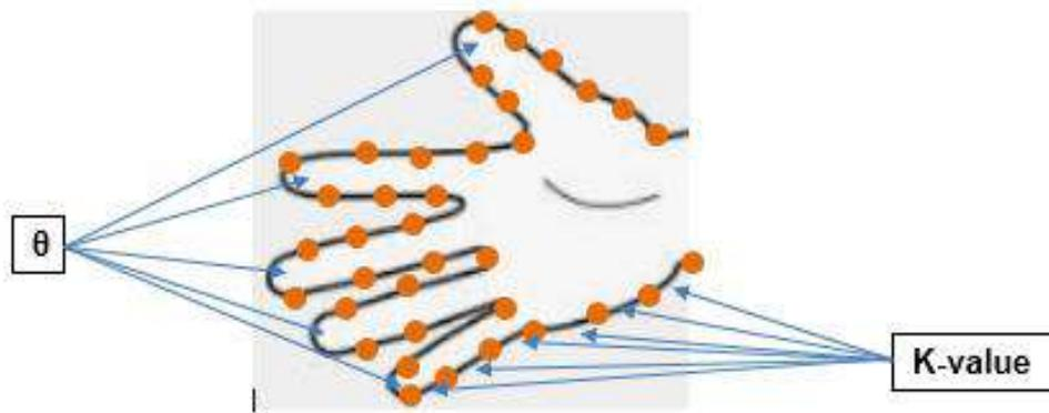
Figure 5.13. K-curvature algorithm with Theta( $\theta$ ) and K value
