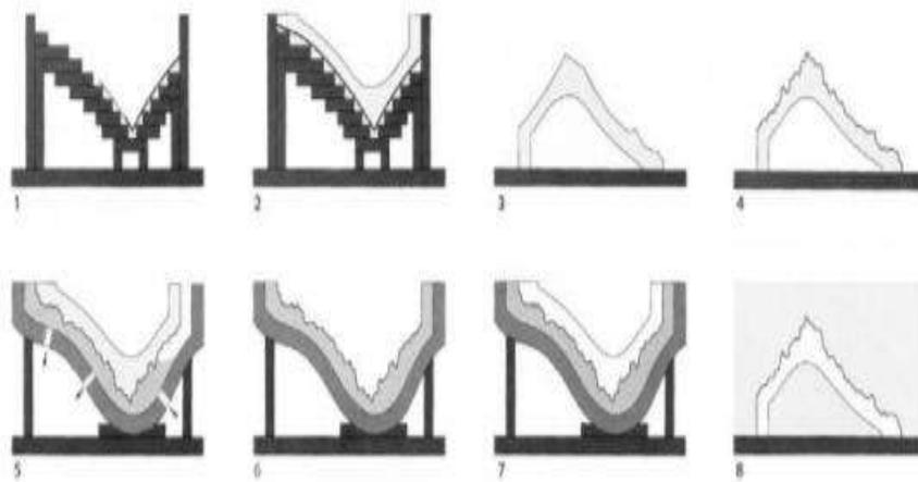
**Figure 2.9.** Building handmade relief model based on Imhof method
