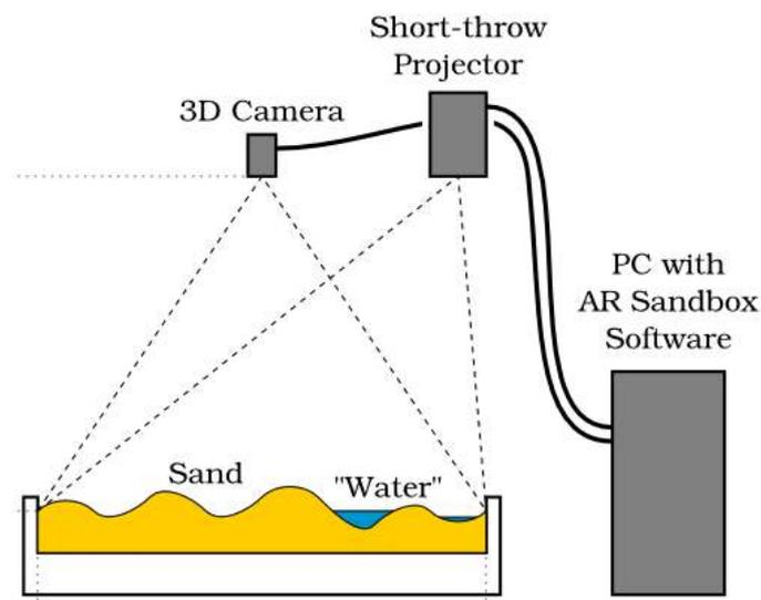
**Figure 5.1.** The typical arrangement of AR Sandbox (Kreylos, O., 2021)
