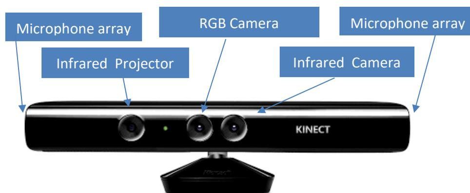
Figure 2.23. Features in Kinect Device
