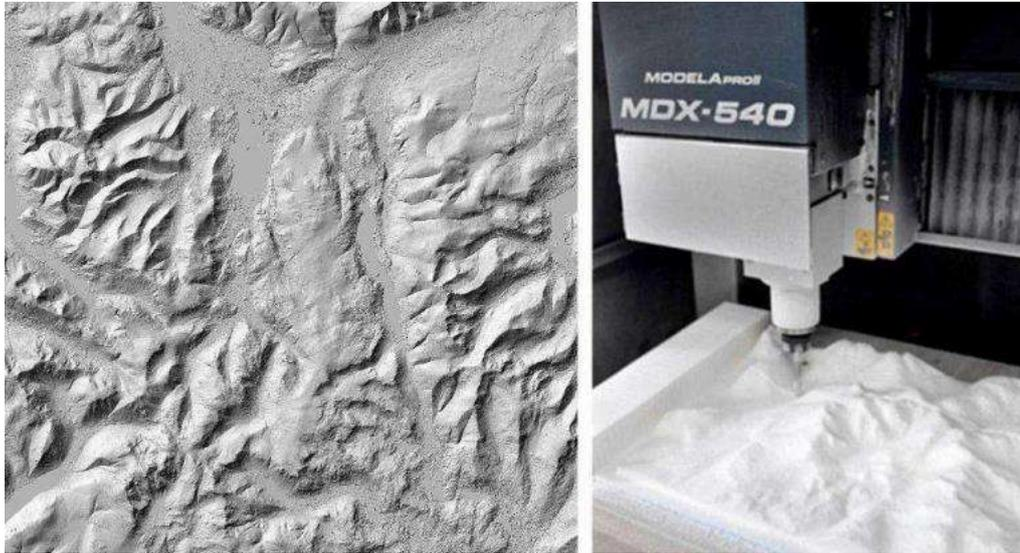
**Figure 2.15.** Generating PARM model and milling process
