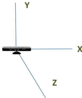
Figure 5.4. Kinect sensor coordinate detection
