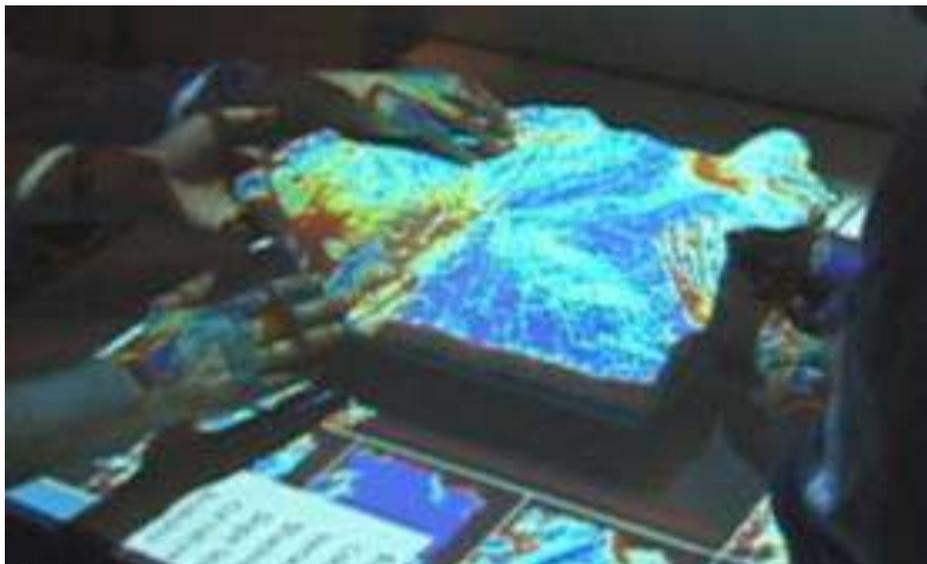
**Figure 2.20.** The projecting of slope variation onto the Illuminating Clay
