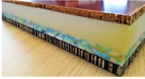
Figure 1.2: Multi-layered structure with composite materials and poro-elastic foams.
